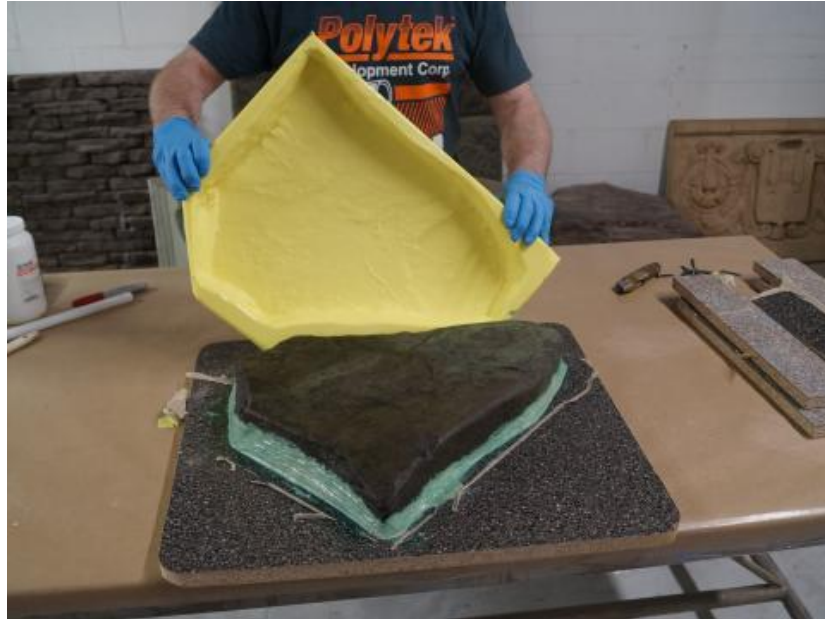
Figure 8: Finished rubber mold of stone to be used for pathway installation (Polytek Development Corp., n.d.)
