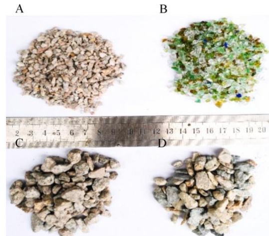
Figure 17. Size differences between fine (above) and coarse (below) aggregates (Chandratilake, 2012)
