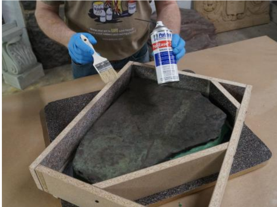
Figure 7: Framework for making a rubber mold of a stone (Polytek Development Corp., n.d.)
