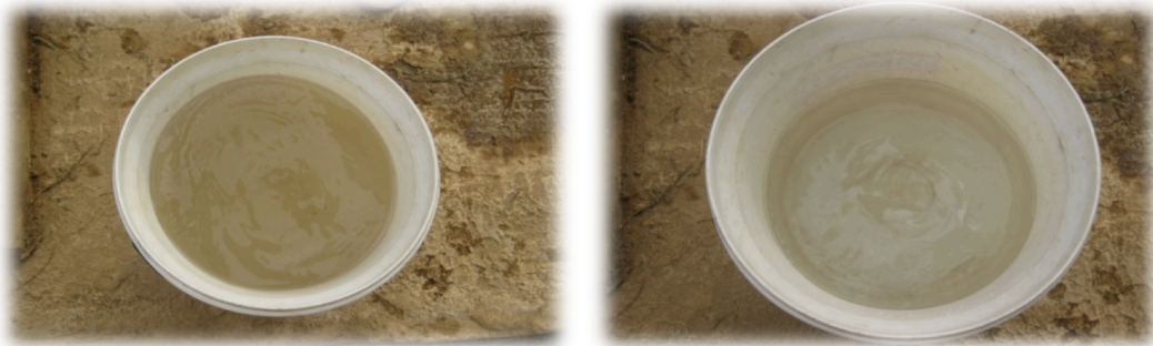
Figure 18. Water before entering the filtration system (left) and after exiting the filtration system through the incentive (right)
