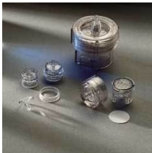
Figure 12. Nucleopore® membrane holder used for urine filtration (Optics Planet 2010).
