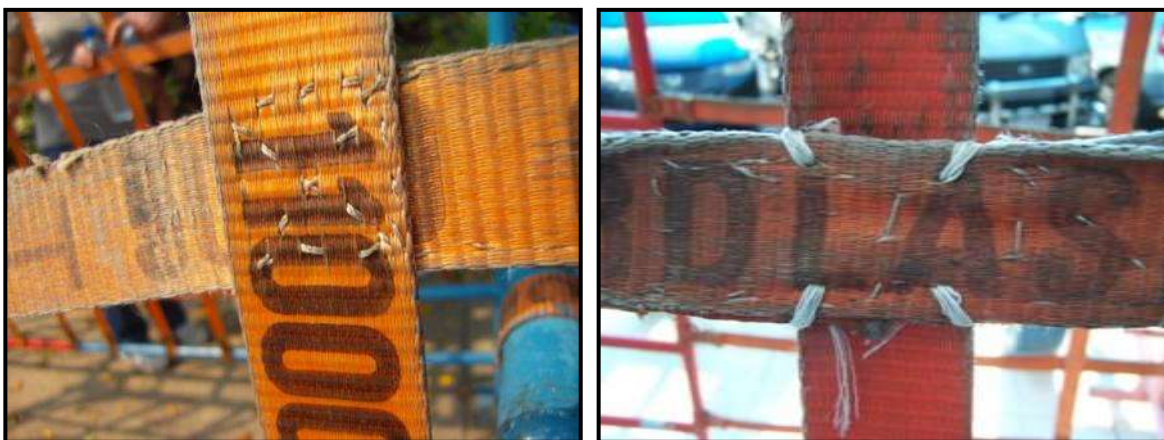
Figure 16. Square stitching method (left) and corner stitching method (right) for stitching tow straps together.
