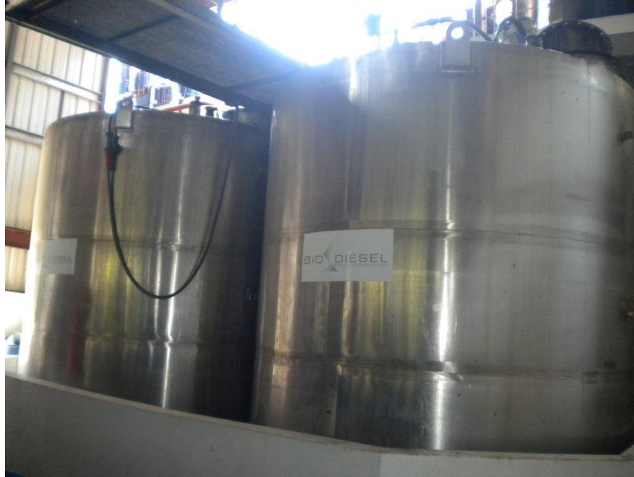
Figure 1 Biodiesel Facility in Guaynabo. The two pressurized tanks produce 50,000 gal. of biodiesel per year.
