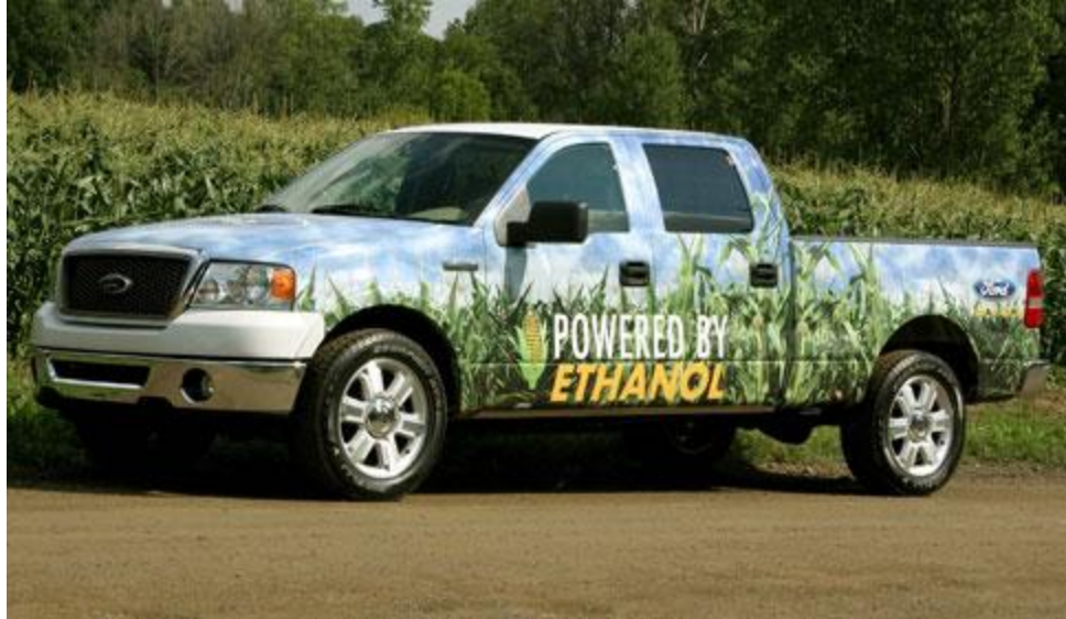
Figure 2 Ford 150 Flexible Fuel Truck. This is one of Ford's FFVs capable of using up to 85% ethanol as a fuel source. It produces fewer emissions when compared to a conventional combustion engine (Siuru, 2007).
