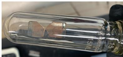
**Figure A.1.** Qualitative representation of what good product yield looks like for  $\text{Cs}_2\text{TiBr}_6$  thin-films deposited on FTO glass.
