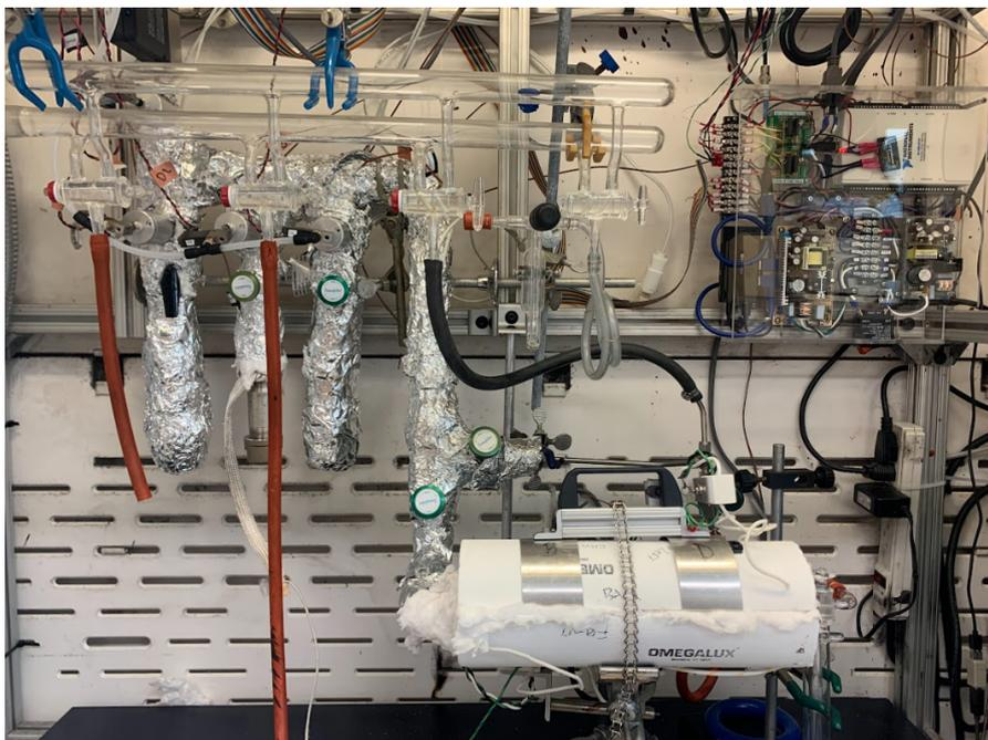
**Figure B.1.** Atomic layer depositor with metal precursors, electronics board, schlenk-line inside the lab fume hood.
