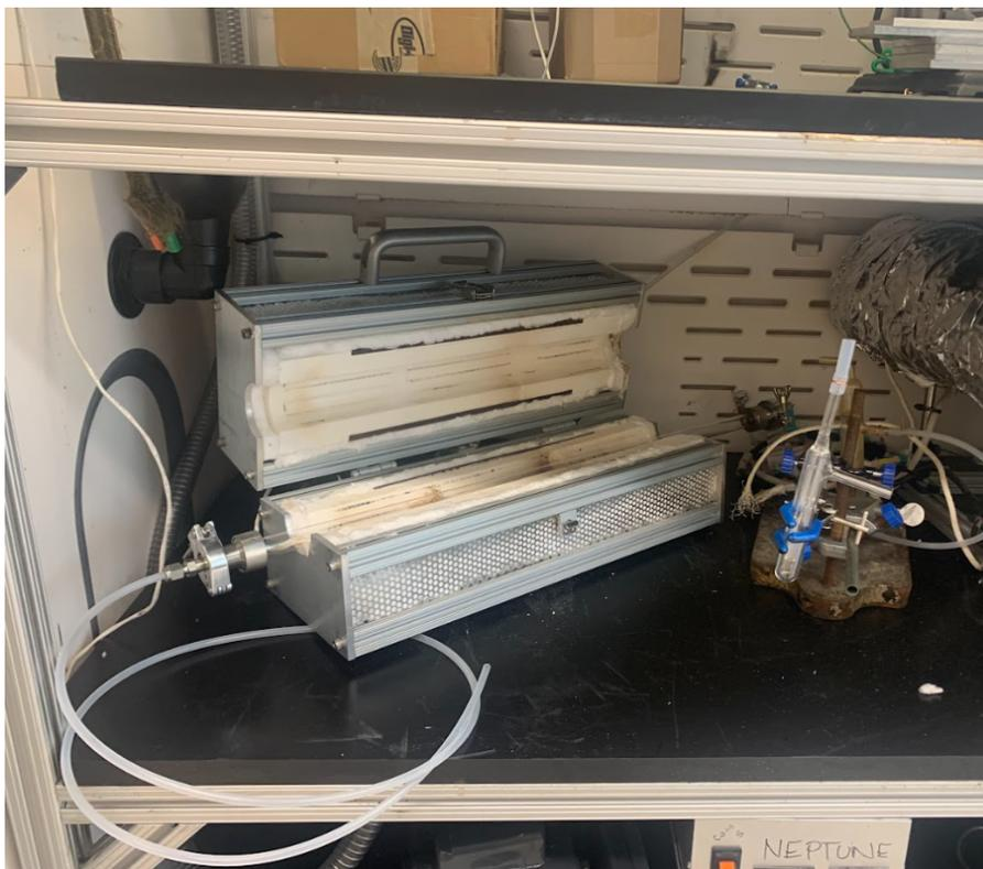
**Figure B.2.** Forming gas apparatus constructed for the realignment of  $\text{Nb}_2\text{O}_5$  ultra-thin layers on the wafers surface. The pictured state does not have the plastic tubing running through the oil bubbler.
