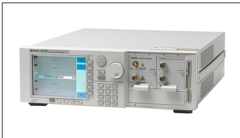
Figure 25: Our Keysight 8164B lightwave measurement system holds a laser source with a range of 1450 nm – 1650 nm [64].
