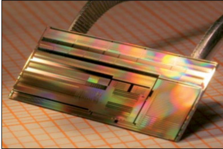
Figure 8: Silicon-on-Insulator chip with a variety of structures including Mach-Zehnder-modulators, Raman-lasers and -amplifiers, Fabry-Pérot modulators, waveguides [41]. Silicon-on Insulator PICs are one of several platforms for PICs.
