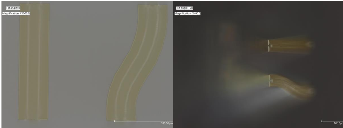
Figure 52: Print 3. The top view (left figure) shows that the waveguide has no height mismatch and the full structure was printed. The side view (right figure) shows that all three parts of the structure (pedestal, ridge, waveguide) are all printed and seem to be without significantly noticeable errors.
