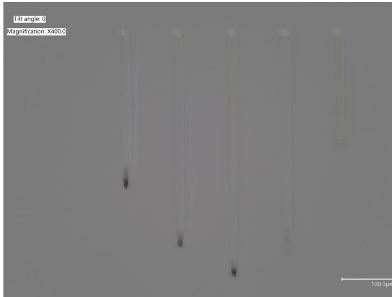
Figure 50: Print 1. Notice the circular path outlined by the edges near the bottom of the figure in addition to the seemingly burnt edges for the left three waveguides. This print failed due to improper block stitch settings.
