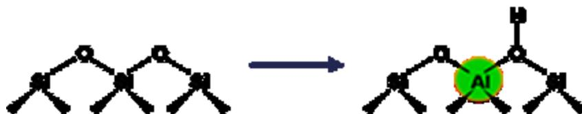
Figure 11 - The formation of acidic site when aluminum hydrogen pair is introduced in zeolite ("Methanol to Olefins," 2017)
