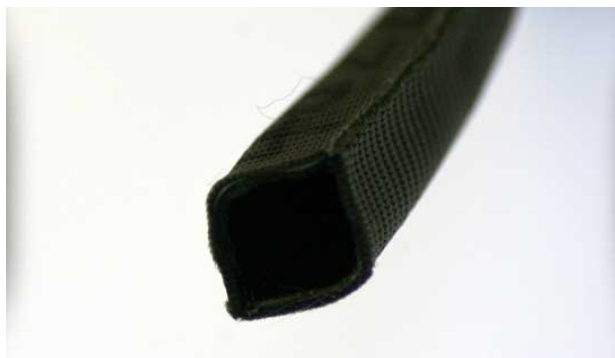
Figure 4.16: Nylon tubular webbing is an excellent sheathing material for hydro-muscles.
