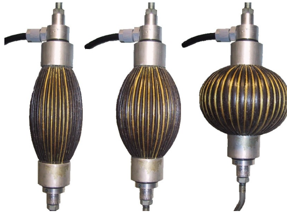
Figure 4.10: McKibben Muscle relaxed/unpressurized (Left) to contracted/pressurized (Right)
