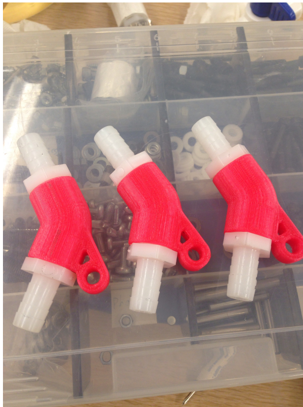
Figure 4.18: The 3D printed components served as fluid inlets as well as mechanical attachment points for the hydro-muscles.
