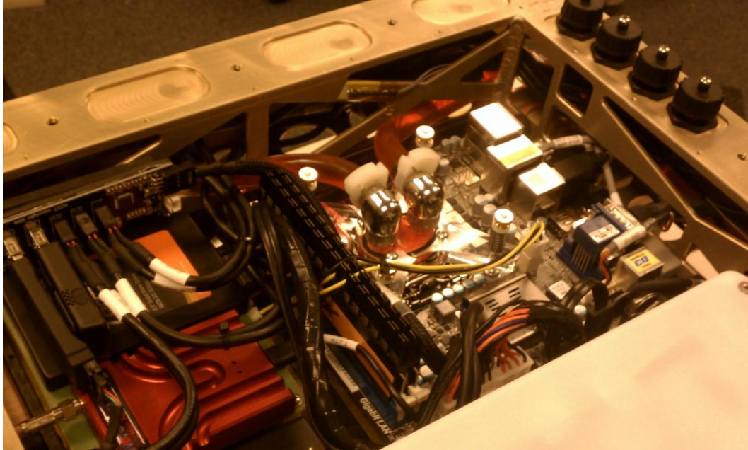
Figure 29: Mini-ITX Motherboard and Water-Cooling System in Rover
