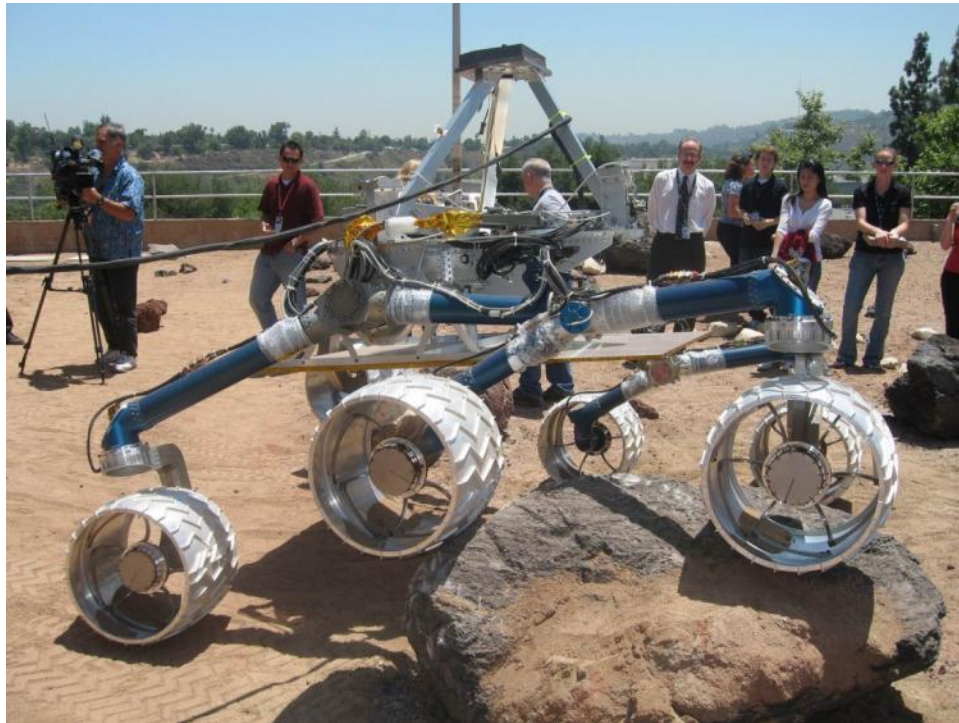
Figure 11: MSL Mobility Prototype on JPL's Mars Yard
