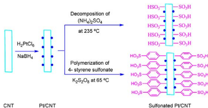
Fig. 2.44 Schematic illustration of two sulfonation routes for Pt/CNT catalysts: (a) decomposition of ammonia sulfonate (b) in situ radical polymerization of 4-styrenesulfonate [8].
