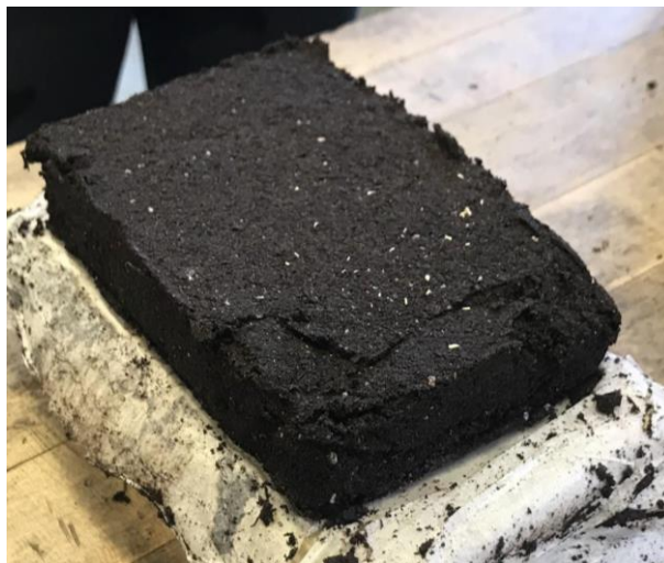
Sample block produced from first mold, with removal deformations (Desmarais, 2021).
