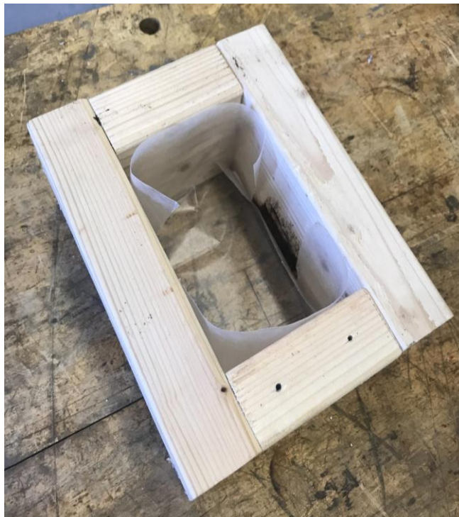
Completed fabrication of first mold design lined with wax paper (Desmarais, 2021).
