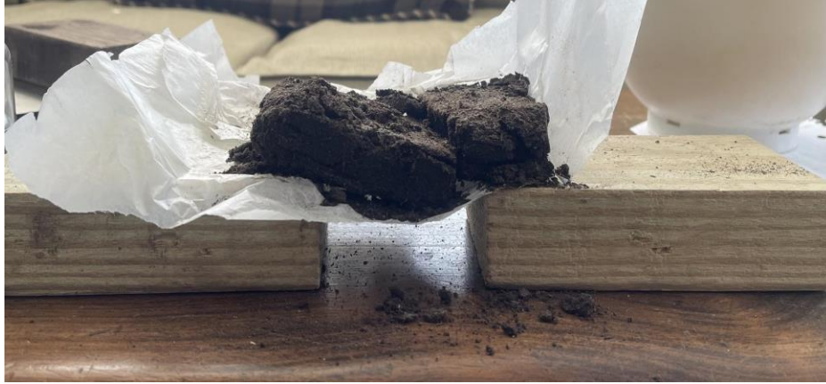
Figure 2. Control UCEB at Failure during Flexural Strength Test (Desmarais, 2021)
