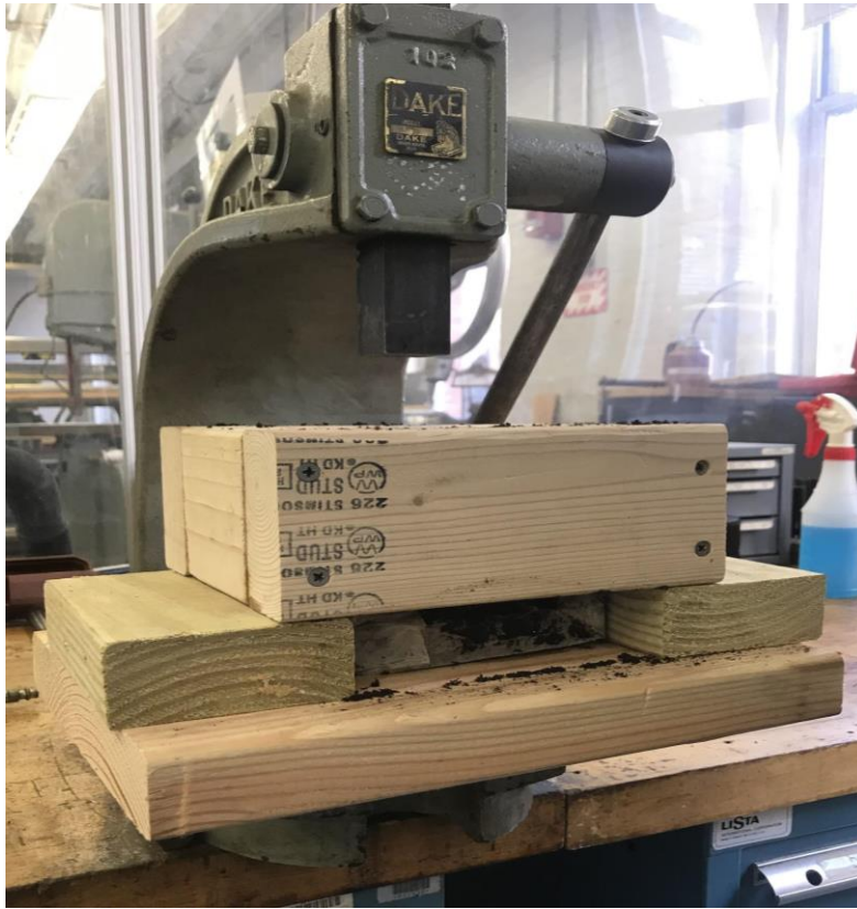
First Mold on Stilts, Finished Block Pressed Out of Mold Collar (Desmarais, 2021).
