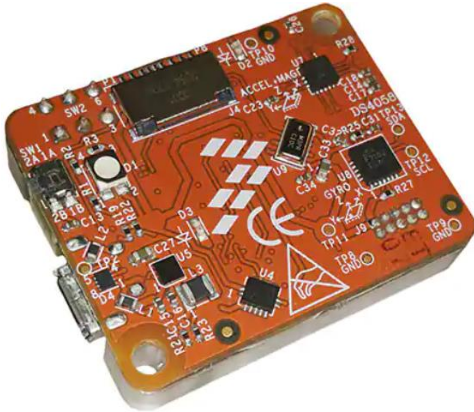
Figure 29 RD KL25-AGMP01 data collection board (Freescale Semiconductor) ©2015, NXP
