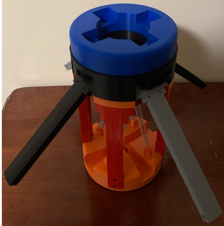
Figure 32 Air Brake Bay Separated and Joined with Air Brakes Deployed
