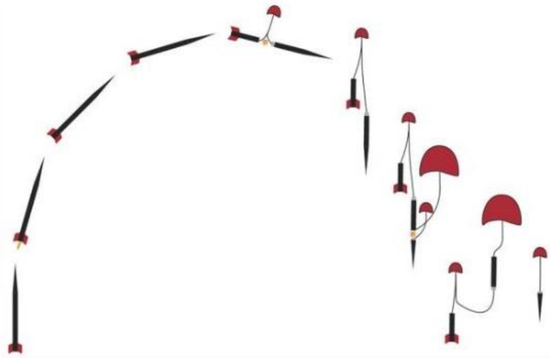
Figure 19 Illustration of Parachute Recovery © WPI Rocket MQP 2019-2020
