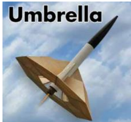
Figure 20 Drag Recovery © Apogee Rockets, 2009
