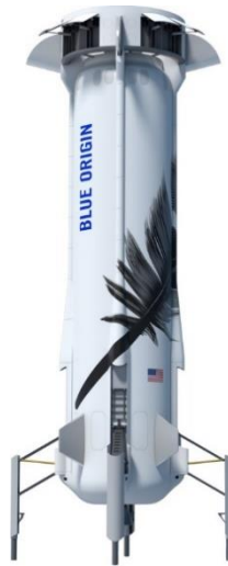
Figure 23 Blue Origin’s New Sheppard Reusable Rocket Booster. © Blue Origin 2019
