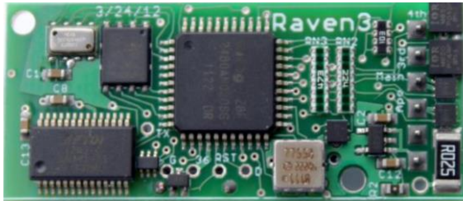
Figure 28 Raven 3.0 Altimeter (Featherweight Altimeters) ©, FA 2009
