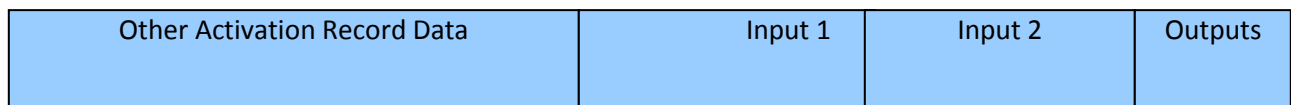
Figure 5.3 - A different perspective on the slab in the slab allocator. Input 1 and Input 2 are pointers to outputs of another activation record(block)
