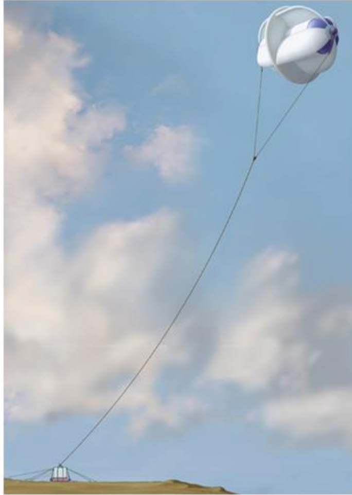
Figure 3.1.9: Image of Magenn rotating helium filled balloon.
