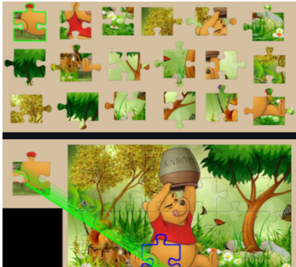
Figure 19: Puzzle piece match displayed by highlighting the location of the piece from the user inputted image and the matching location on the puzzle. The matching keypoints contributing to this match are connected with lines
