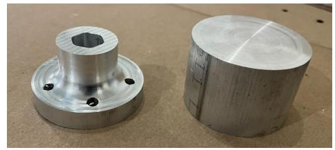
Figure 65. Machined Wheel Hub & Stock.
