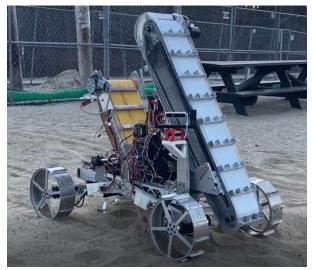
Figure 119. Robot in Depositing Configuration.
