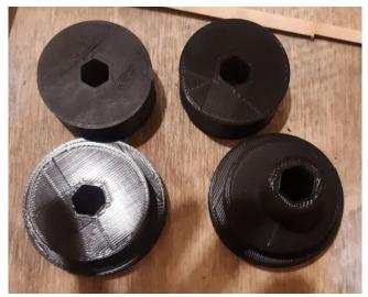
Figure 83. 3D-printed Pulleys for Storage Conveyor Rollers.
