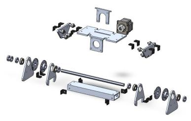
Figure 81. Exploded View of Conveyor Rotational System.
