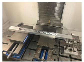
Figure 62. Frame Component after Lightening Operation in VM-2.
