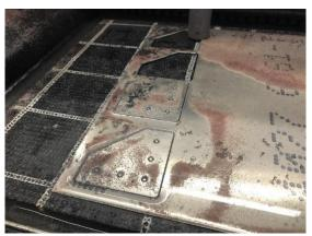
Figure 63. Triangle Brackets in Wazer Waterjet.
