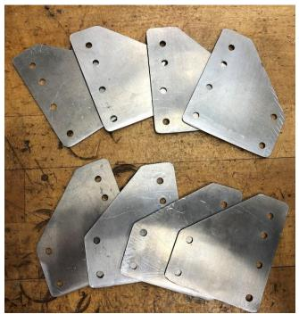
Figure 64. Motor Mount Brackets.
