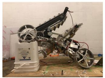
Figure 116. Robot Traversing 40 cm Obstacle.
