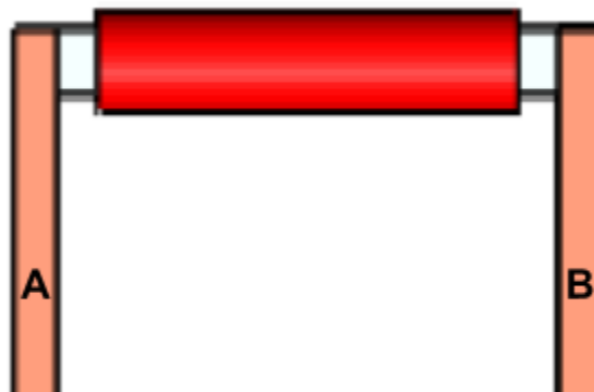
Figure 20: Top View of Cantilever with Piezoelectric Strips Labeled
