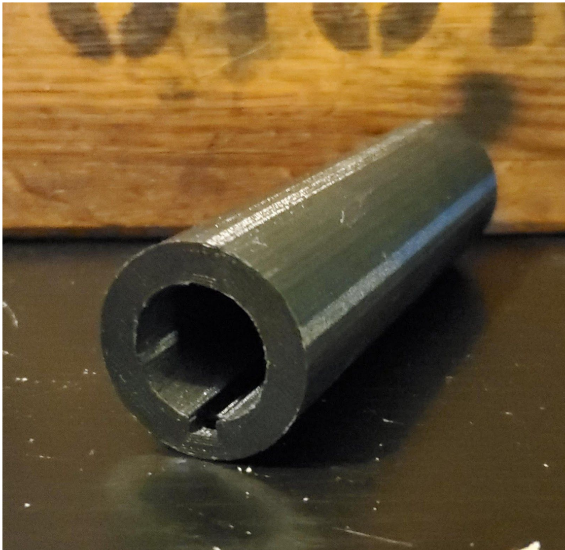
Figure C6: Prototype Adapter for Driveshaft
