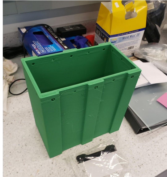
Figure B1: Battery Housing Initial 3D-Printed Prototype Bottom
