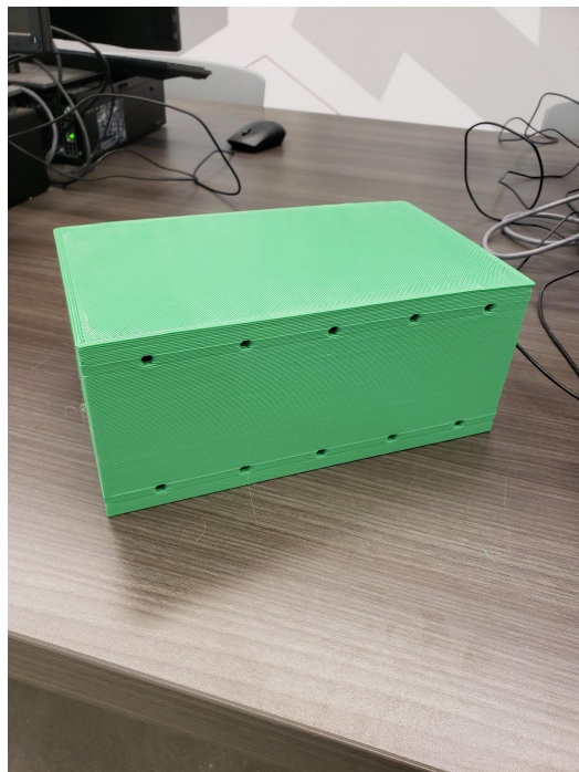
Figure B2: Battery Housing Initial 3D-Printed Prototype Top
