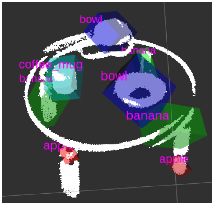
Figure 2.5: Visualization of predicted labels for objects in scene
