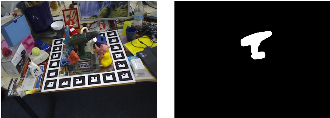
Figure 3.4: An RGB Image and a binary mask inferred from Segmentation network
