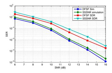
Figure 6.13: Symbol error rates for multipath channel.
