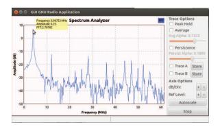
Figure 5.12: View of the spectrum analyzer application in GNU Radio. The GUI shows the signal sampled from the ADC and processed to be compatible with the GNU Radio environment. In this picture we see a frequency domain plot of the signal with a measured frequency of 3.96753MHz MHz
