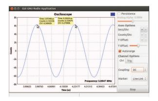
Figure 5.11: View of the oscilloscope application in GNU Radio. The GUI shows the signal sampled from the ADC and processed to be compatible with the GNU Radio environment. In this figure, we see a time domain plot of the signal with a measured frequency of 3.9447 MHz
