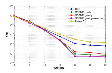
Figure 3.14: Bit error rate curves for the Vehicular A channel
