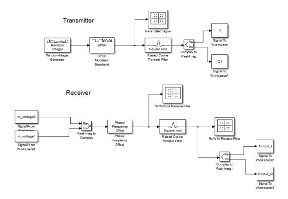
Figure 6.11: Pre-processing required for experiment. At the top we have the pre-processing that occurs in the transmission. At the bottom we have the pre-processing in the reception.
