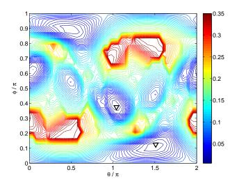
Figure 3.5: Contours of BER for a three-tap unit norm filter, parameterized by two angles in spherical coordinates. The  $\bigtriangledown$  indicates the filters with the lowest BER.
