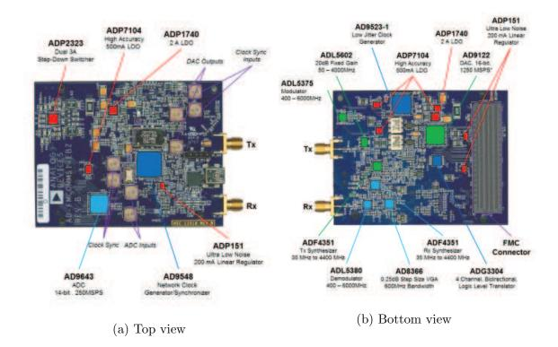
Figure 5.1: The FMCOMMS1 module is a RF front-end (RFFE) board. Here we have the board and markers highlighting important components of the platform, such as the ADC, DAC, (de)modulators and amplifiers. Source: [4], used with permission.
