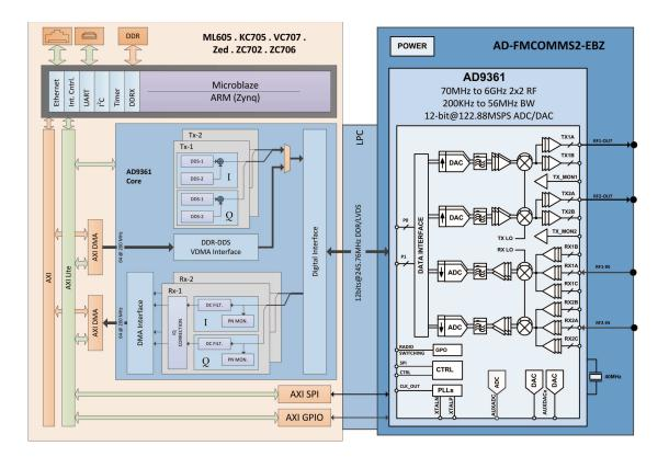
Figure 5.5: Schematic of the software-defined radio hardware. On left, we have the FPGA development board and on right we have the FMCOMMS2 RF Front-End. The figure illustrates the transmit and receive chain. Source: [5], used with permission.
