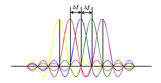
Figure 2.5: Orthogonal subcarriers in a OFDM scheme. The subcarriers are separated by a  $\Delta f$  frequency spacing.
