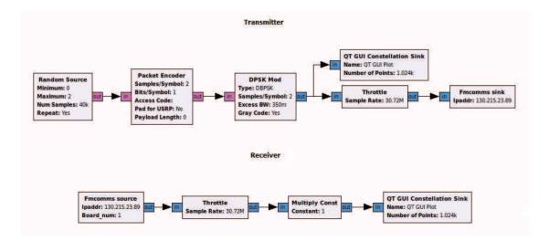
Figure 5.16: Transmitter and Receiver configurations in GNU Radio. The signal is generated and modulated in DBPSK symbols before being sent to the "Fmcomms sink". The signal goes through the transmitting and receiving paths in the hard-ware platform and the received I/Q are delivered back to GNU Radio through the "Fmcomms source" block.
