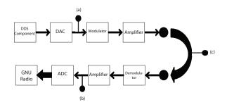
Figure 5.8: Experiment Set-Up. The points (a), (b) and (c) show the probing positions for the obtained measured signals in the Results subsection
