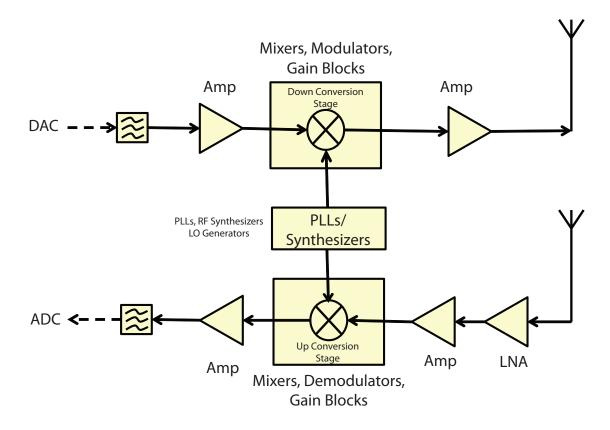
Figure 2.10: Block diagram of a typical RF Front-End. In the transmitter path, the the analog signal is modulated and transmitted in RF frequencies. In the receiver path, the analog high-frequency signal is converted to baseband before being processed by the ADC. The local oscillator (LO) drives both transmitter and receiver circuits.
