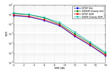
Figure 6.7: Symbol error rates for vehicular channel.
