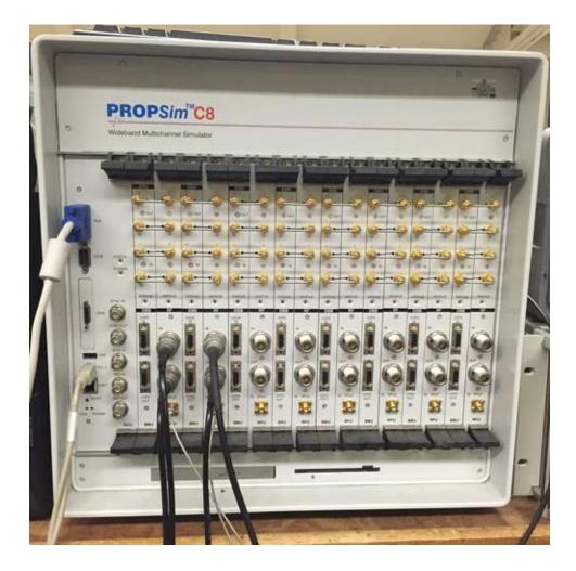
Figure 6.9: PropSim channel emulator at the Center for Wireless Information Network (CWIN) Lab.
