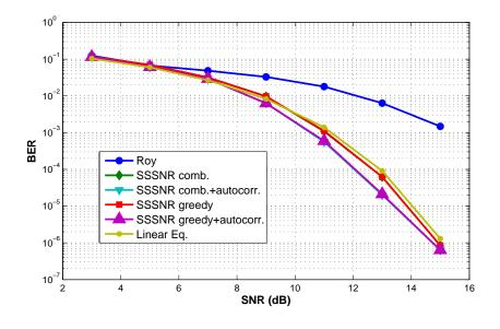
Figure 3.11: Bit error rate for same CSF design metrics shown in 3.10 plus the addition of the squared autocorrelation penalizing term.
