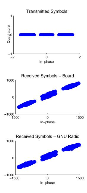
Figure 5.17: Transmitted and received DBPSK symbols sent through the platform. The transmitted symbols are generated and modulated in GNU Radio and sent through the transmit chain. The symbols are then fed back to the receive chain and can be visualized using the ADI IIO oscilloscope tool in the ZedBoard and inside the GNU Radio environment.
