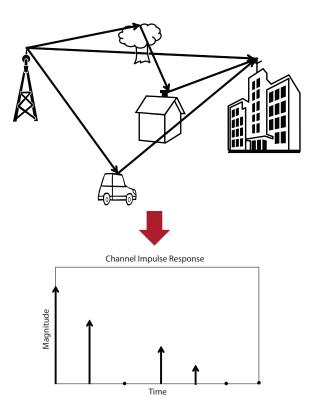
Figure 1.2: Intersymbol interference phenomenon forming the channel delay profile
