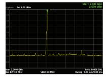
(c) Frequency Response of the RF signal obtained with a spectrum analyzer. The measure point is indicated as (c) in Fig. 5.8
