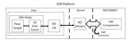
Figure 5.7: High level illustration of the onboard transmitting/receiving processes. The sink/source blocks in GNU Radio communicate with the IIO drivers inside the same platform.
