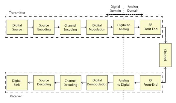
Figure 2.9: Block Diagram showing the Digital and Analog divide in a Software-Defined Radio Platform. The digital signal processing is performed in the digital domain in baseband, while the analog portion of the system performs the RF operations. Based on [3], Figure 5.
