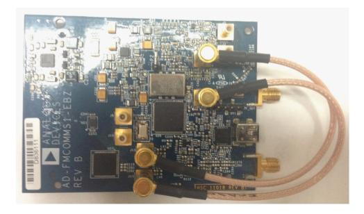
Figure 6.3: FMCOMMS1 board in baseband configuration. The output of the DAC is connected to the input of the ADC using SMB cables.
