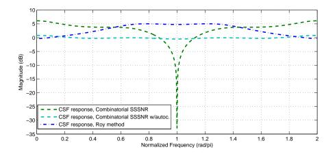
Figure 3.12: CSF frequency response for combinatorial, combinatorial with addition of penalizing term, and Roy's approach.
