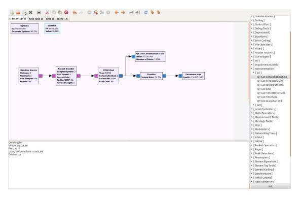
Figure 2.11: The GNU Radio Companion (GRC) tool. It allows design of communication systems using pre-made and custom blocks.
