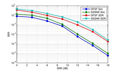
Figure 6.14: Symbol error rates for vehicular channel.
