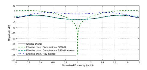
Figure 3.13: Frequency response of original channel and effective channel frequency responses for combinatorial, combinatorial with addition of penalizing term, and Roy's approach.
