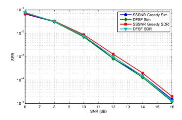
Figure 6.6: Symbol error rates for multipath channel.
