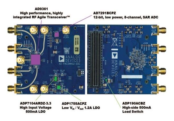
Figure 5.2: The FMCOMMS2 is a high-speed analog module designed by Analog Devices. Source: [5], used with permission.
