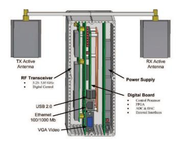
Figure 2.8: The KUAR radio. Source: [2]
