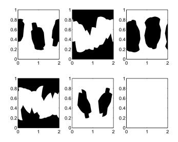
Figure 3.4: Usage maps of the 6 taps of the effective channel **c**. Axes are identical to Fig. 3.2. Dark areas indicate that the given tap is one of the  $\mu$  largest taps in **c**.
