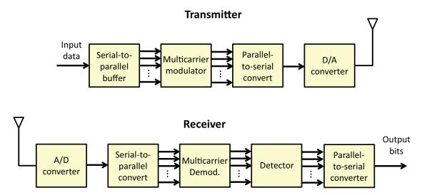
Figure 2.4: Block diagram representing a multicarrier transmission system. For the transmission, the information is first parallelized to be modulated and in the receiver, the information is also parallelized to be demodulated and detected.
