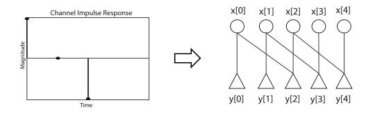
Figure 2.2: The  $h = \begin{bmatrix} 1 & 0 & -1 \end{bmatrix}$  channel represented as a factor graph. The graph is formed by bit nodes, which are the channel inputs (x[.]) and the check nodes, which are the channel outputs (y[.]). The connections between bit nodes and check nodes represent the dependencies between the received and transmitted symbols.
