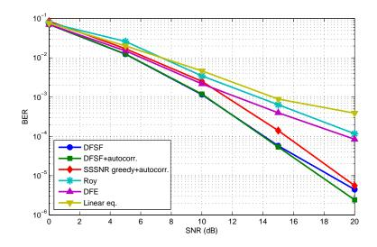
Figure 4.3: Bit error rates for the Vehicular A channel
