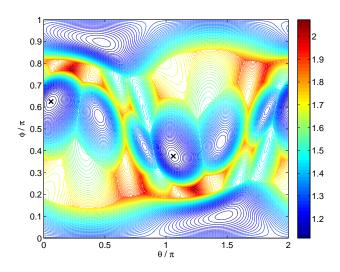
Figure 3.2: Contours of SSSNR for a three-tap unit norm filter, parameterized by two angles in spherical coordinates. The  $\times$  indicates the filter with the highest SSSNR.
