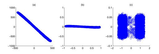
Figure 6.12: The received BPSK symbols. In (a) the received constellation collected from the ADC's buffer. In (b) we have the constellation after the phase compesantion and in (c) after the square root raised cosine filter.
