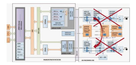
Figure 6.2: Schematics for the baseband experiment with the FMCOMMS1 board. The RF portion of the board is disconnected from the DAC and ADC outputs and the signal is redirected to go from the DAC output to the ADC input.
