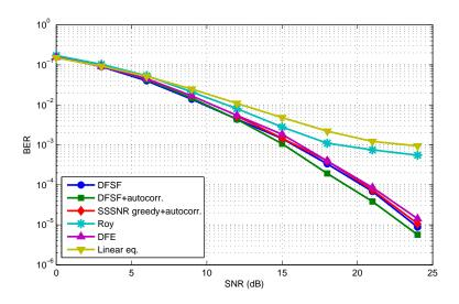
Figure 4.4: Bit error rates for 5-tap channel with equal power delay profile
