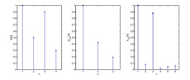
Figure 3.3: Channel, filter, and effective channel tap magnitudes, using the SSSNR-optimal 3-tap filter.
