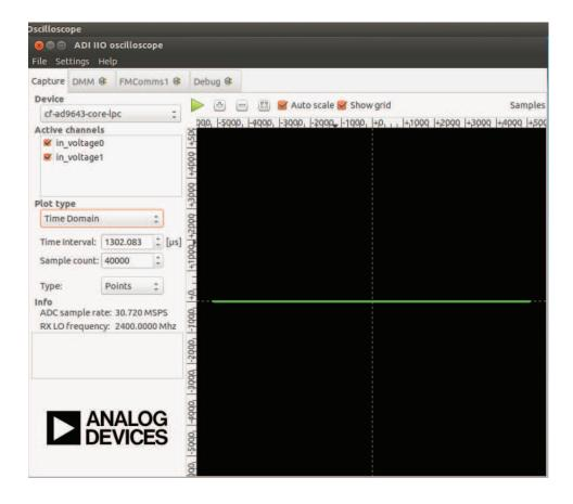
Figure 6.4: The baseband signal received at the ADC. The BPSK symbols are scattered along the X axis making the detection operation unfeasible.
