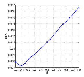
Figure 3.9: Bit error rate as a function of  $\beta$  for the weighted SSSNR scheme
