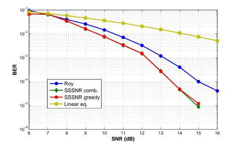
Figure 3.10: Bit error rate for different CSF design metrics
