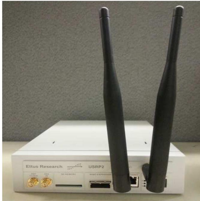
Figure 2.7: The Universal Software Radio Peripheral 2 (USRP2). The software defined radio platform developed by Ettus Research.
