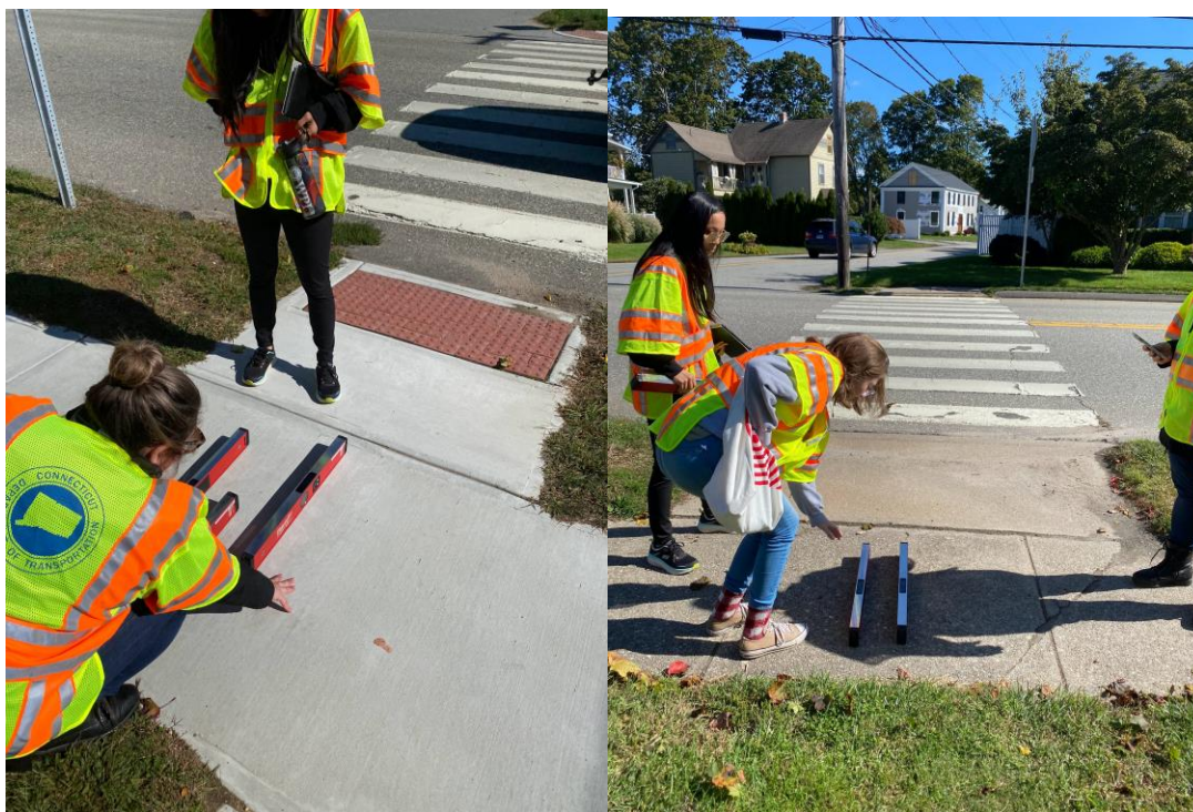
Figure 12: Measuring Curb Ramps During Site Visit
