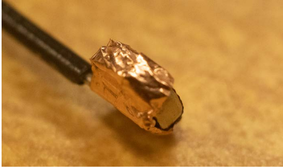
Figure 5.7: Magnet Encased in Copper Foil and Attached to Wire
