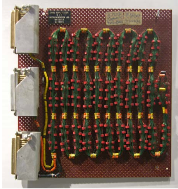
Figure 2.5: Core Rope Memory Test Sample from Apollo Program (Wikimedia Commons 2022)
