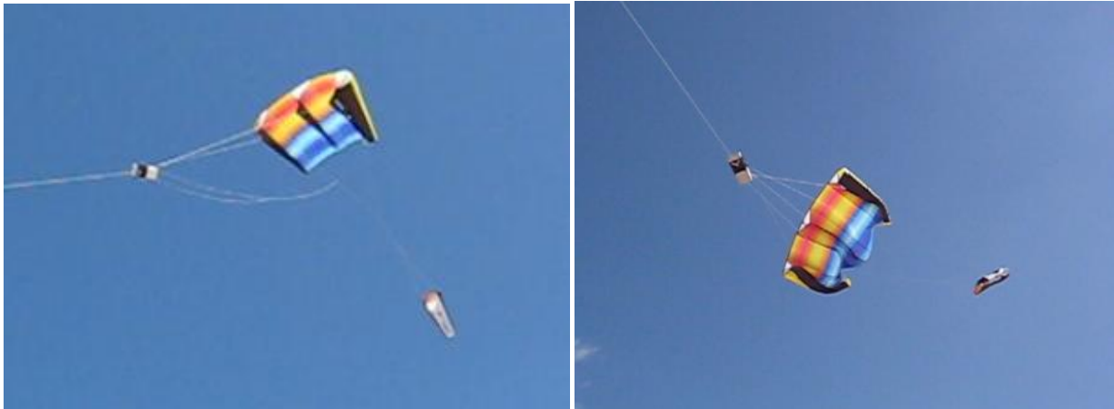
Figure 29: Lifting Kite with Loose TE Lines (Left), and Stalled Kite with Tight TE Lines (Right)
