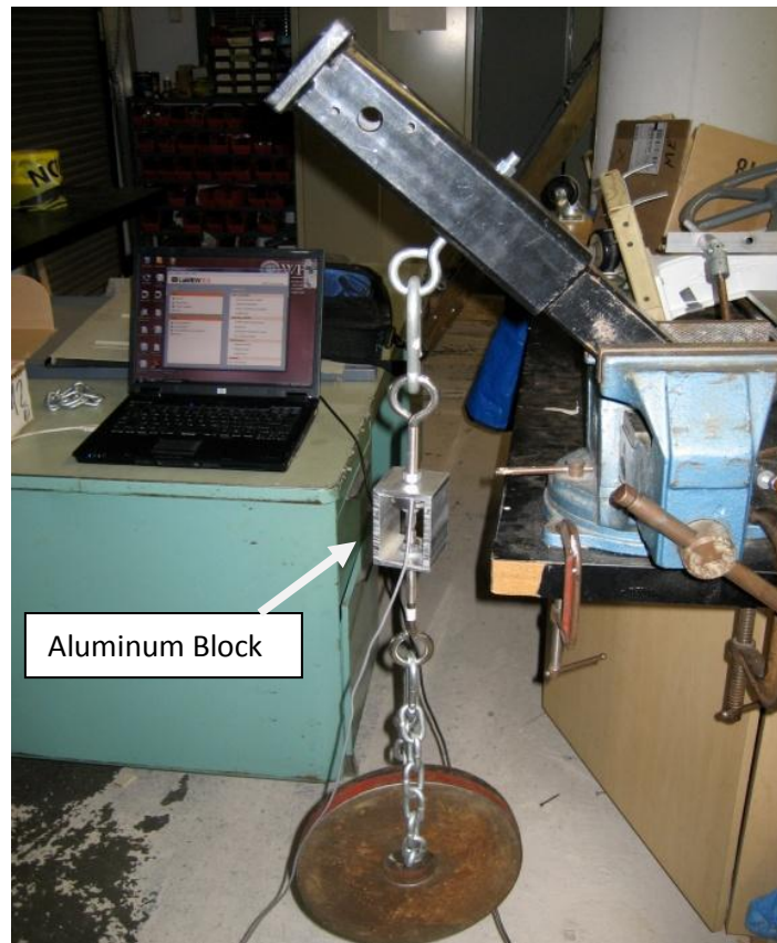
Figure 21: Load Cell Calibration [5]
