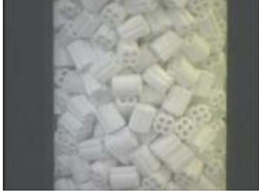
Figure 7. Tube Packed with Steam Reforming Catalyst (Stitt, 2005)
