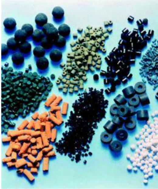
**Figure 2. Example Catalyst Particles (Eigenberger & Ruppel, 2012)**
