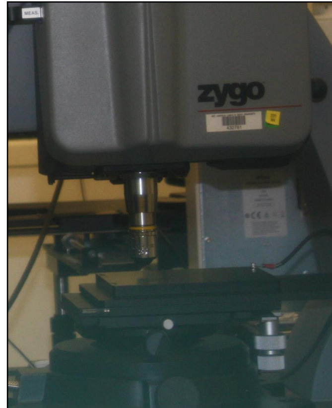
Zygo microscope used to measure surface roughness
