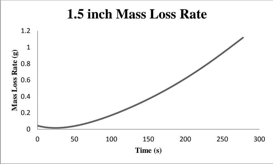
Figure 8: Mass loss rate of fuel in one and half inch inner diameter ice cylinders
