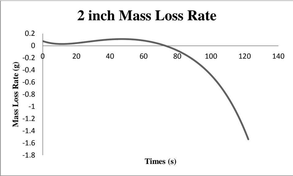
Figure 9: Mass loss rate of fuel in two inch inner diameter ice cylinders
