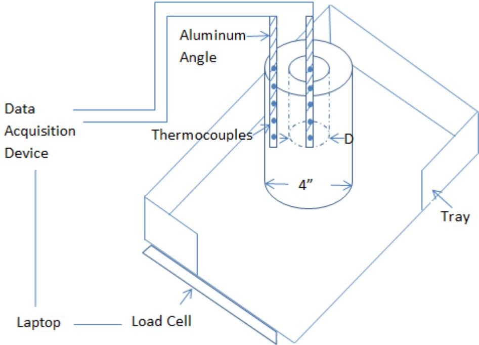
Figure 1: A diagram of the experimental setup
