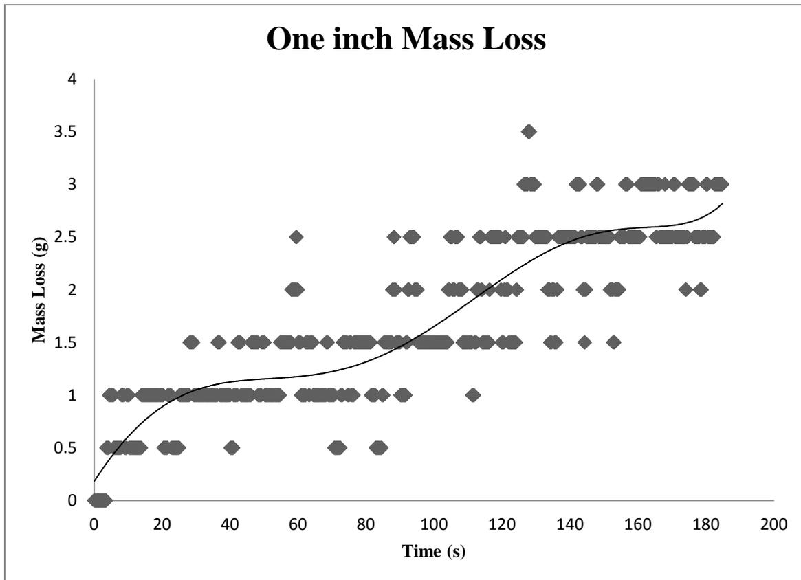
Figure 3: Mass loss of fuel in one inch inner diameter ice cylinders
