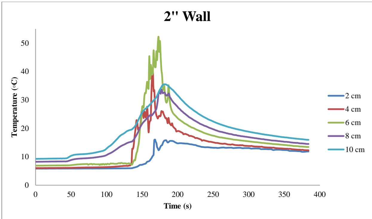
Figure 11: Temperature profile in the ice wall
