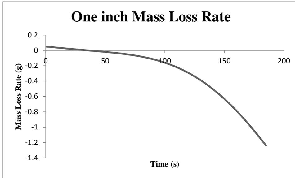
Figure 7: Mass loss rate of fuel in one inch inner diameter ice cylinders
