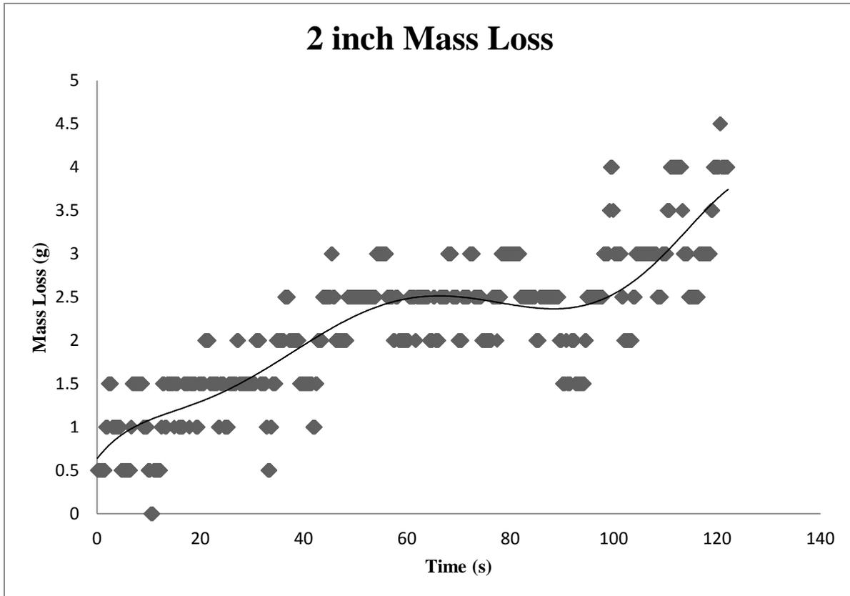
Figure 5: Mass loss of fuel in two inch inner diameter ice cylinders
