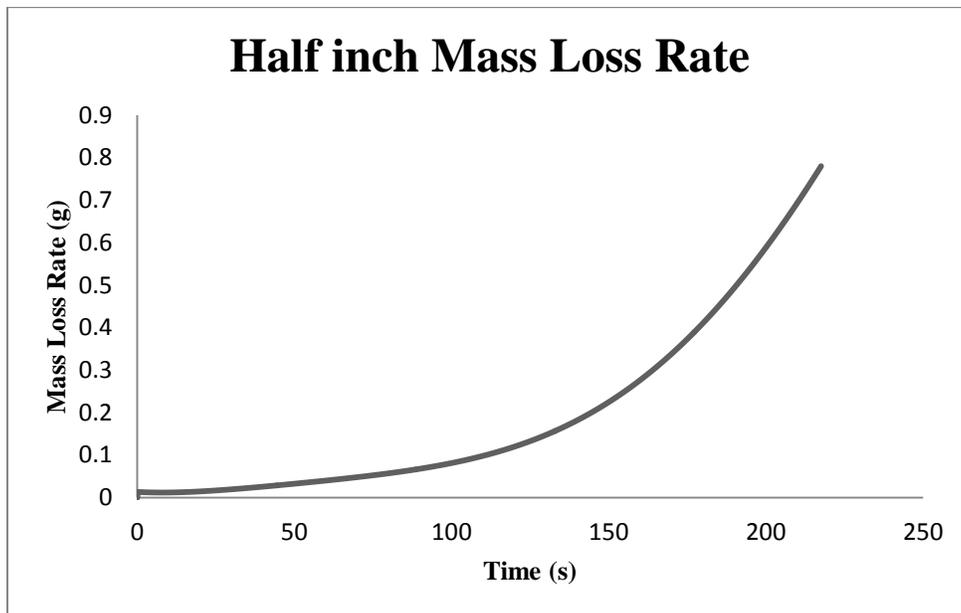
Figure 6: Mass loss rate of fuel in half inch inner diameter ice cylinders
