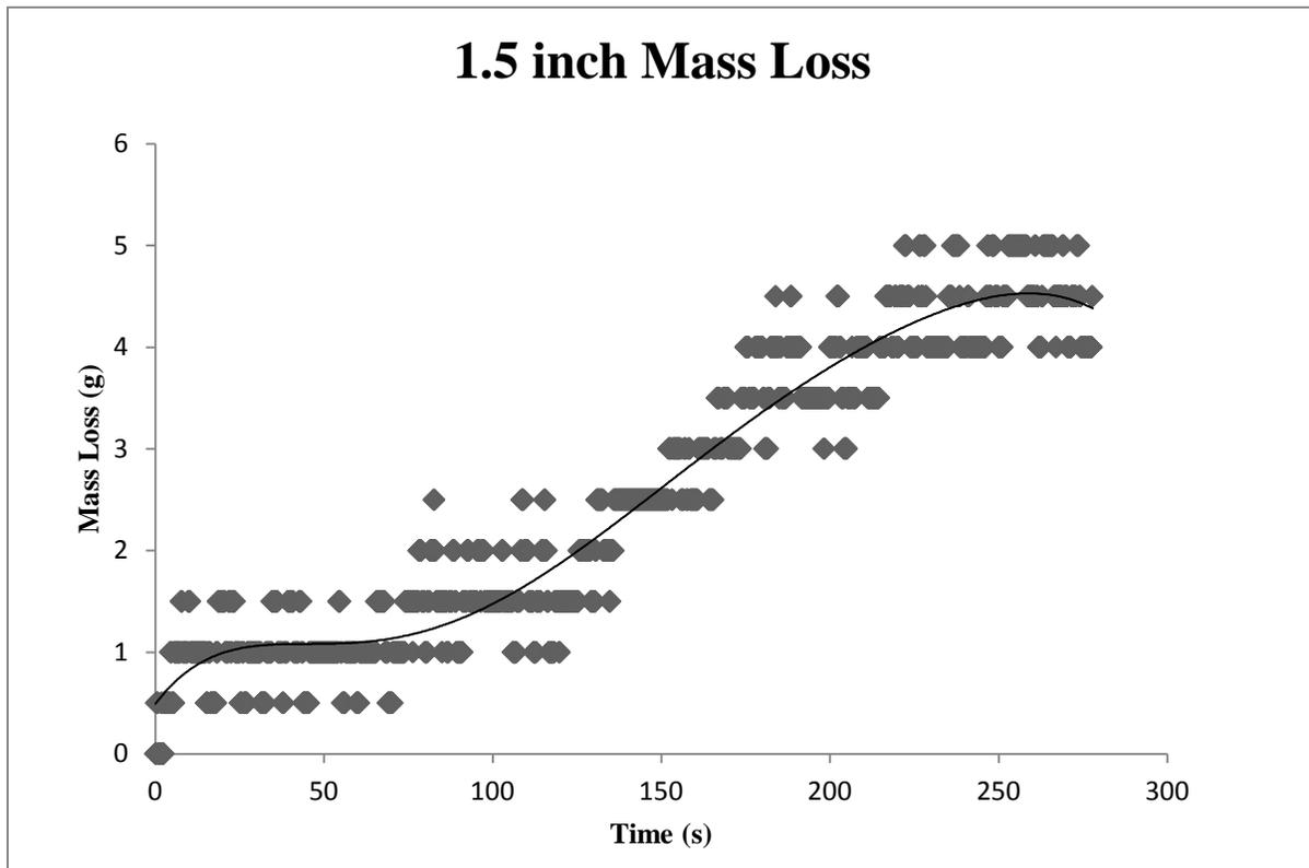
Figure 4: Mass loss of fuel in one and half inch inner diameter ice cylinders
