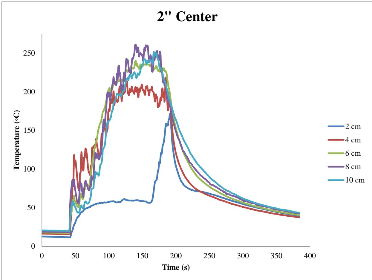
Figure 10: Temperature profile in the center of 2" ice cylinder
