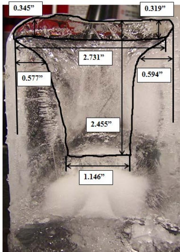
Figure 12: Measurements of an ice cavity with lip
