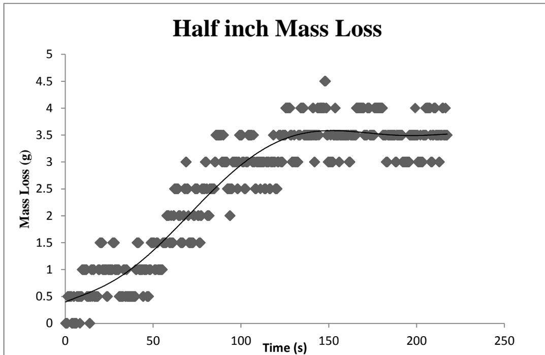
Figure 2: Mass loss of fuel in half inch inner diameter ice cylinders
