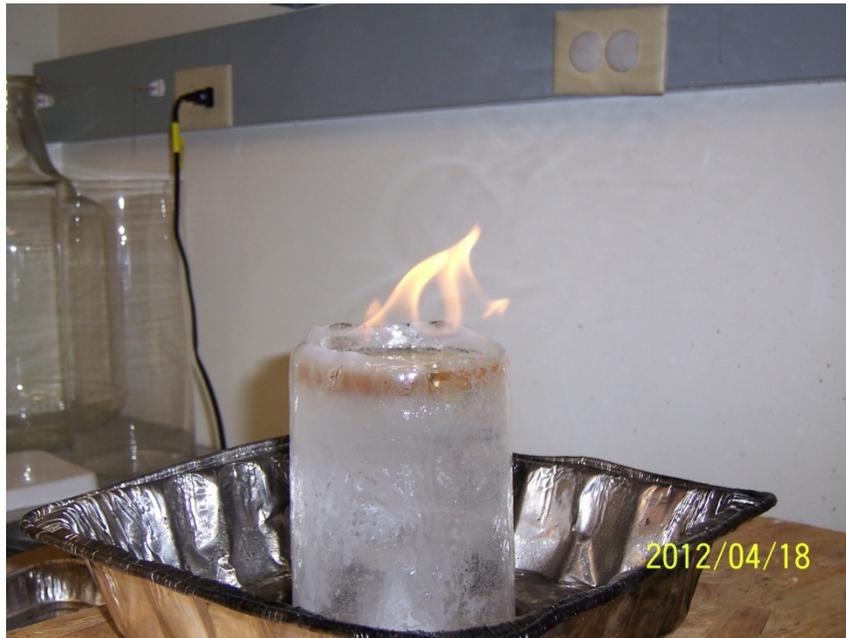
Appendix 1: *In situ* burning of liquid fuel in an ice cylinder
