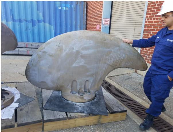
**Figure 7:** One blade from a Controllable Pitch Propeller on a Coast Guard cutter.
