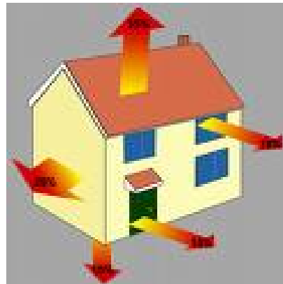
Figure 7: A visual explanation of the ways heat can escape a building (Source: www.energystar.gov )
