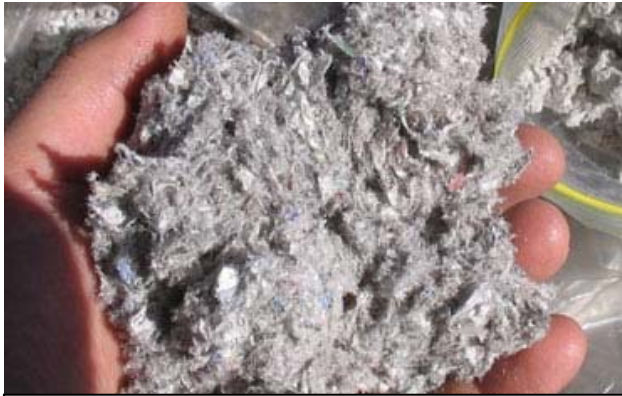
Figure 11: Cellulose is Packed Tightly in Wall Cavities For Insulation (Source: www.inhabitat.com )
