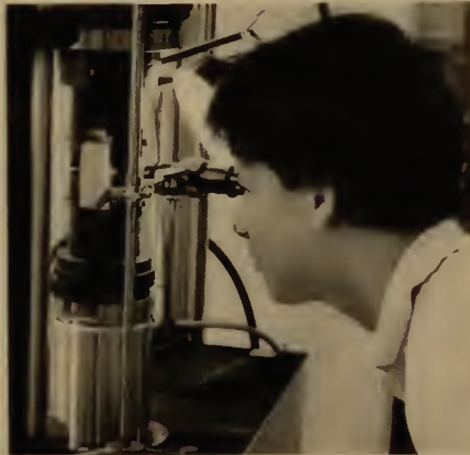
Located in the Arthur E. Smith '33 Materials Processing Laboratory, this Instron servohydraulic, computer-controlled, mechanical testing system evaluates the tension, compression, fatigue and fracture characteristics of metals, ceramics, plastics and other composites.
