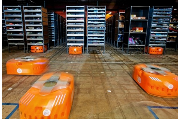
Figure 13: Image of Amazon Robotics system in action. The QR codes are the small white squares on the ground, the robots scan these when they are over top of them and move on from there. [36]
