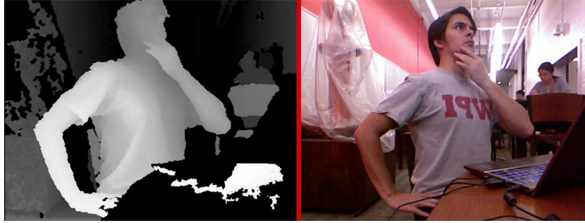
Figure 11: Experimental output depth map of the Xbox Kinect Sensor. The Xbox Kinect calculates the depth by emitting an infrared array of dots, . The left image is the represented depth images outputted by the Xbox Kinect and the right image is the RGB image
