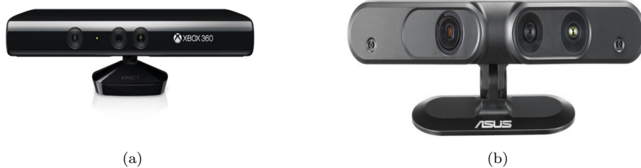
Figure 10: a: The Xbox Kinect b: The Asus Xtion. Both of these sensors are RGB-D sensors, utilizing an infrared dot matrix in its calculation of depth. Note: Images are not to scale. Images courtesy of Microsoft and vr-zone.com, respectively.
