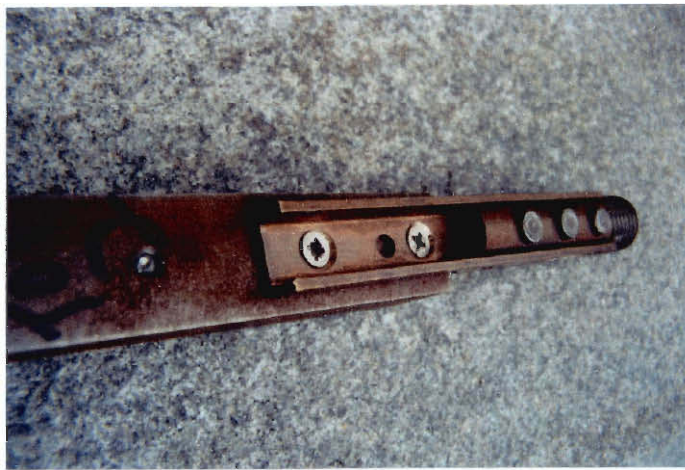
Picture 5: Sheared screw on worn liner
