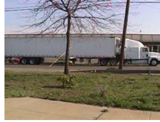
Figure 12 Example of a >T4, a 5-axle truck
