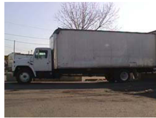
Figure 10 Example of a T2; two-axle truck with 6 tires
