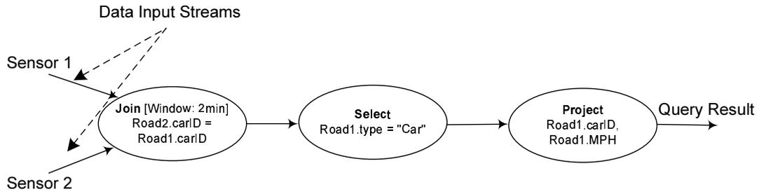
Figure 3.3: Query Plan Constructed from CQL Statement.
