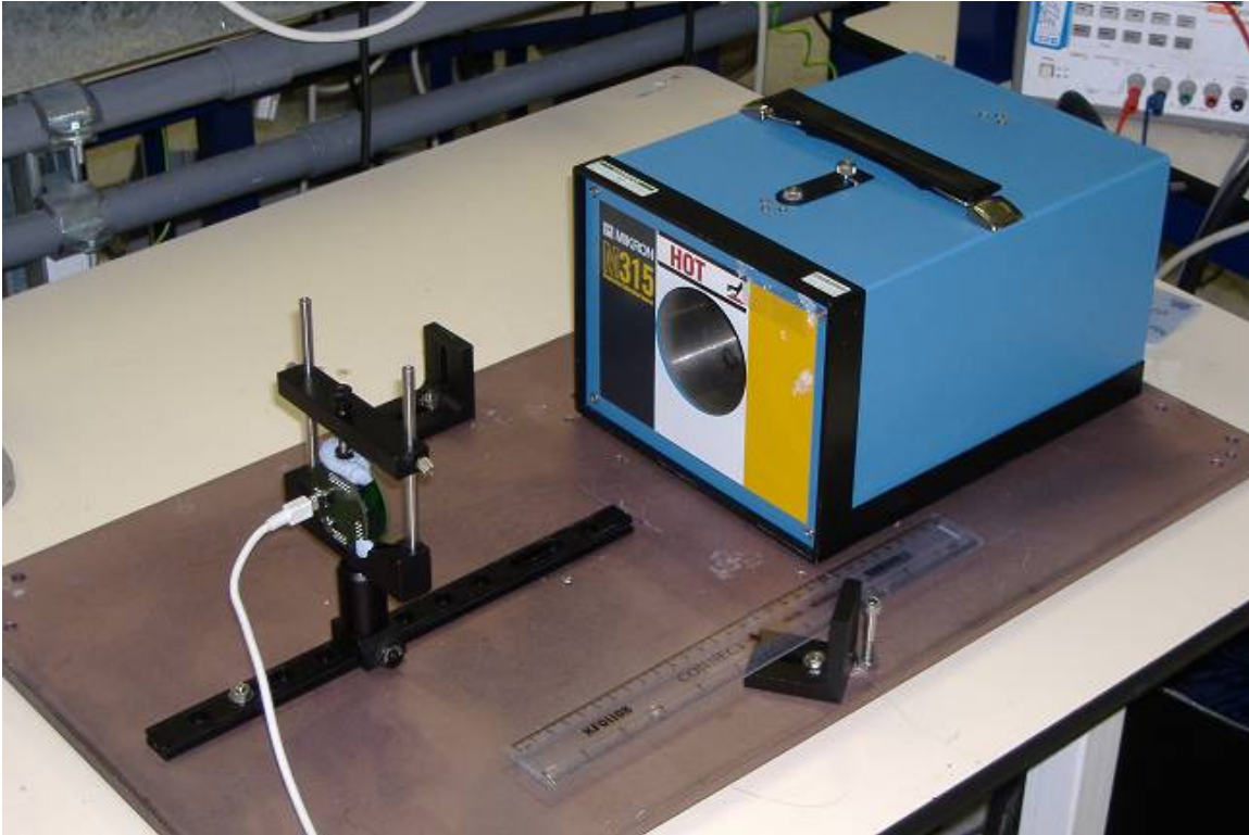
Figure 46: Imaging test with the sensor directly facing the blackbody.
