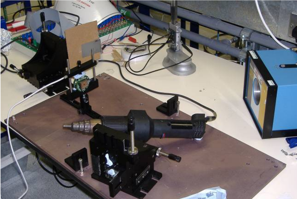
Figure 53: Sensor facing the blackbody source and heat gun (back).
