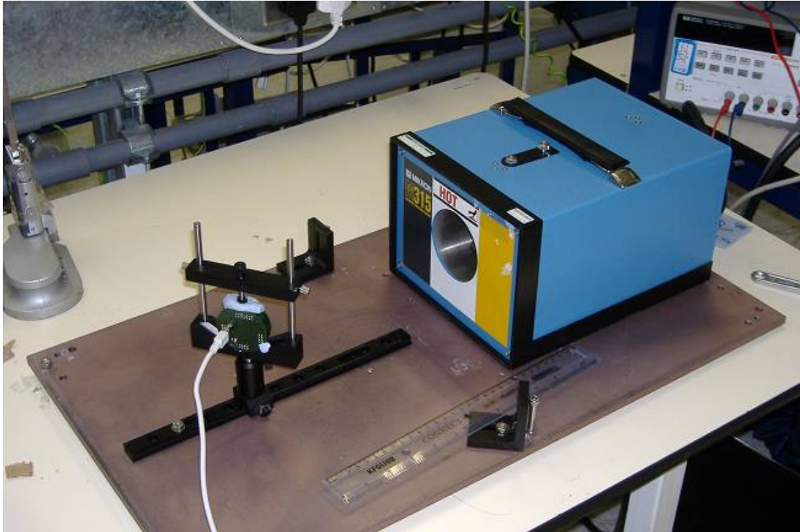
Figure 49: Imaging with the Blackbody to the right of the sensor.
