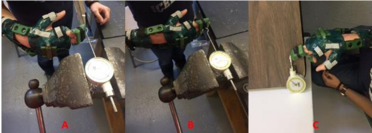
Figure 105: Force Test Setups (A: Attached to Finger Sleeve, B: Attached to Velcro Strap, C: Pushed by Finger)
