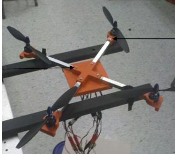
Figure 11: Through Holes on Upper Body and Motor Mounts
