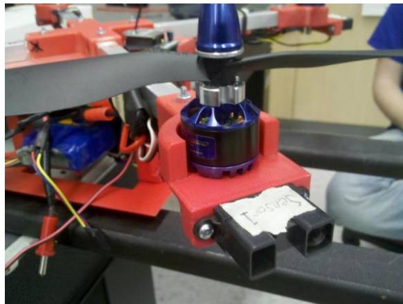
Figure 12: Motor Mount with Motor and IR Sensor Attached
