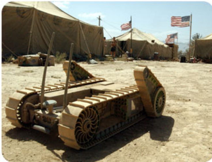
Figure 2 - The Packbot Scout, a battle-tested Unmanned Ground Vehicle (UGV) designed for Military Operations, tested in both Afghanistan and Iraq ( www.irobot.com ).
