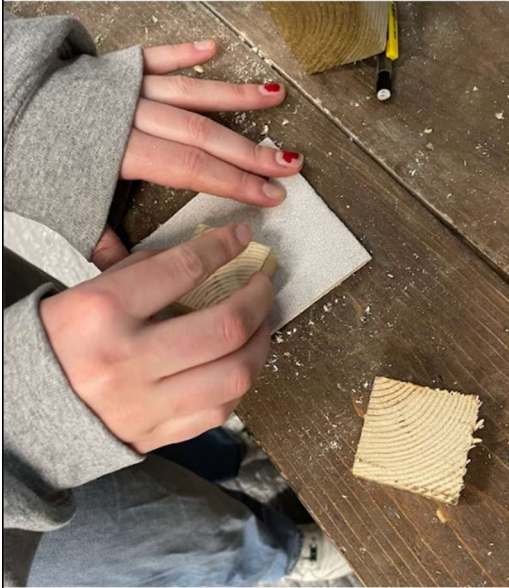
Step 2 Smoothing out the wood edges and splinters
