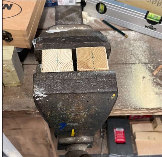
Step 6 Preparing the wood for drilling.
