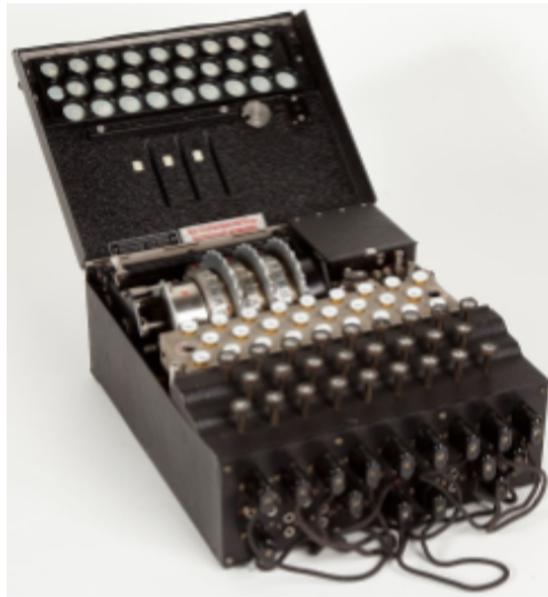
Fig 10: A three rotor variation of an Enigma Machine
