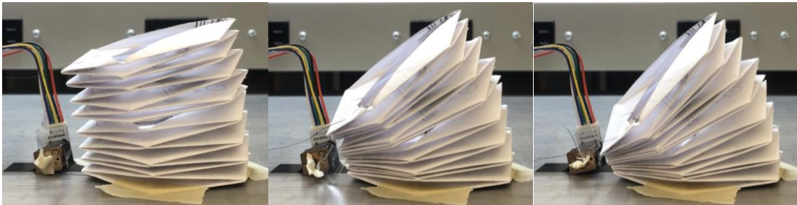
Figure 14: Progression of Yoshimura collapsing.
