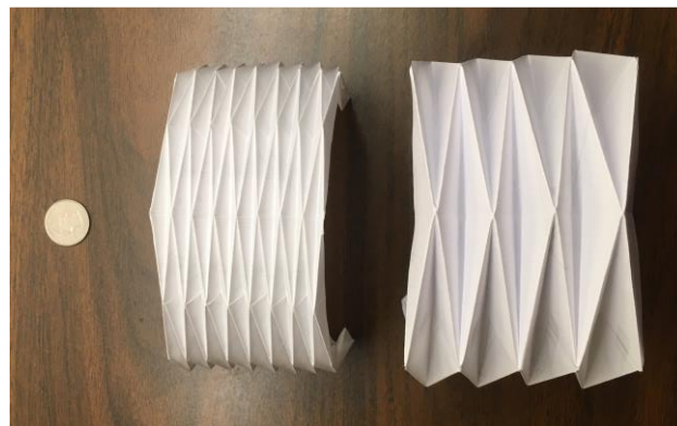
Figure 11: Yoshimura pattern with different radial frequencies and axial lengths.
