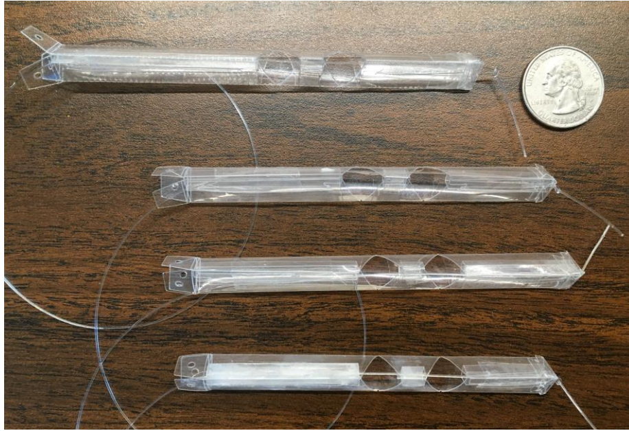
Figure 16: Triangular beam design with optimized link length from Votta et al.
