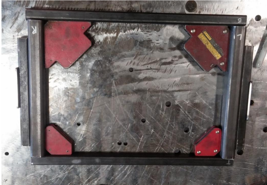
Figure 72: Seat Frame Ready for Welding
