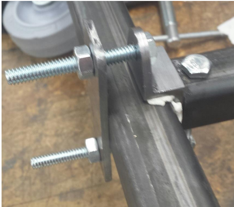
Figure 69: Crossbeam Attachment to Side Frame
