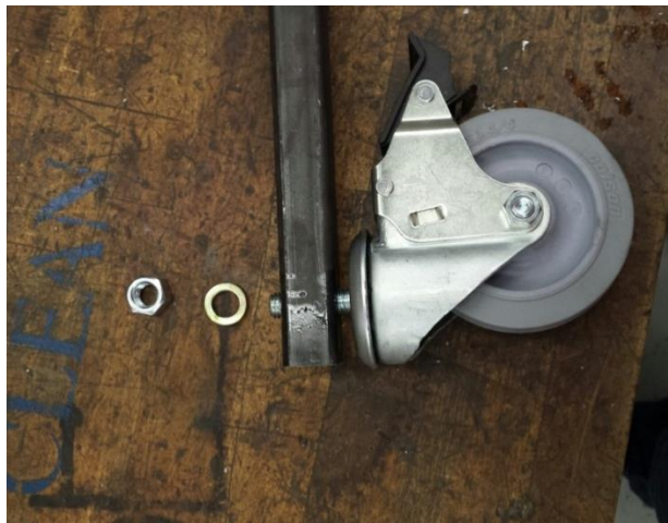
Figure 65: Exploded view of Caster Sub-Assembly
