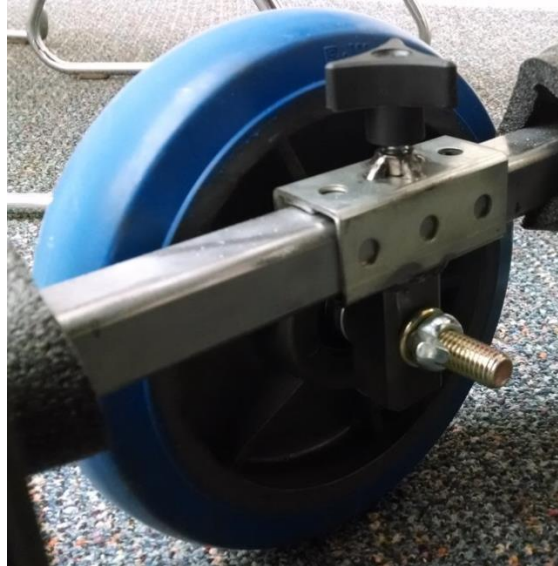
Figure 75: Axle Wheel Attachment
