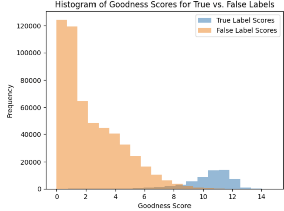
Figure 13: Post-training histogram of networks goodness scores, depicting a clear separation between true (blue) and false (orange) label scores, demonstrating the network’s ability to learn.
