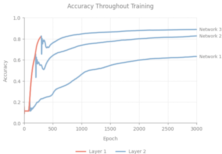
Figure 24: Plot of the performance for three neural networks that differ in the training duration of their first hidden layer. It highlights the network’s learning progress and shows the relationship between the first hidden layers’ training length and the following learning. The graph provides insight into finding an optimal training duration for the first layer that supports a productive learning progression without diminishing the value added by later layers.
