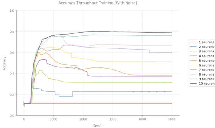
Figure 20: A comparative analysis of neural network performances with noise added to the data employs the same neuron count configurations as in Figure 19. This chart highlights the changes in test accuracy caused by increased data complexity, showing a general decline in performance across all configurations.
