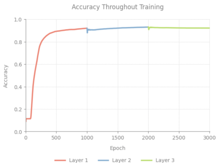
Figure 11: Chart showing the training accuracy of a neural network trained using the FF algorithm across three layers of 500 neurons. The accuracy quickly peaks during the initial training phase and remains consistently high across subsequent layers through 3000 epochs.
