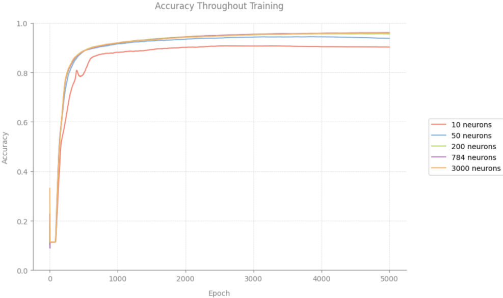
Figure 18: The graph compares the evolution of network accuracy over a training period of 5000 epochs for five networks. Each network has a single hidden layer with varying neuron counts, ranging from 10 to 3000 neurons.
