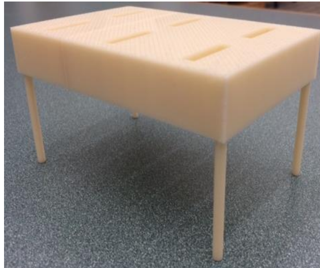
Figure 32: Picture of the rapid prototyped glass slide holder.
