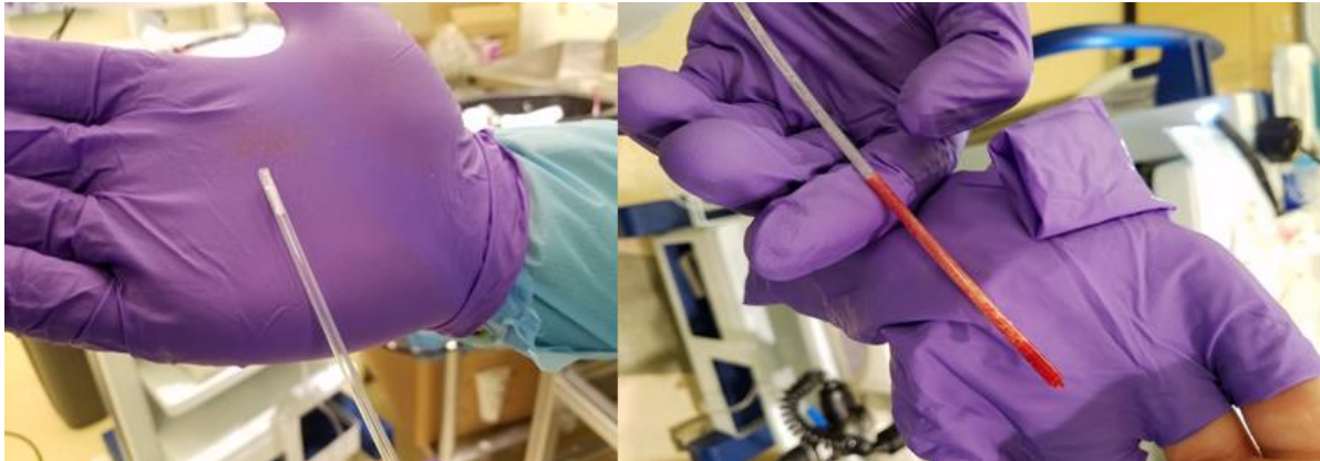
Figure 20. Catheter and PCL plug on the left and the right image shows the clogged catheter post removal.
