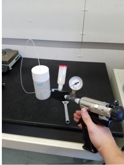
Figure 21. In this image, the common setup for spray tests is shown. Not shown is the source of compressed air. The quick connect provides connection from the catheter to the “Black Block.”
