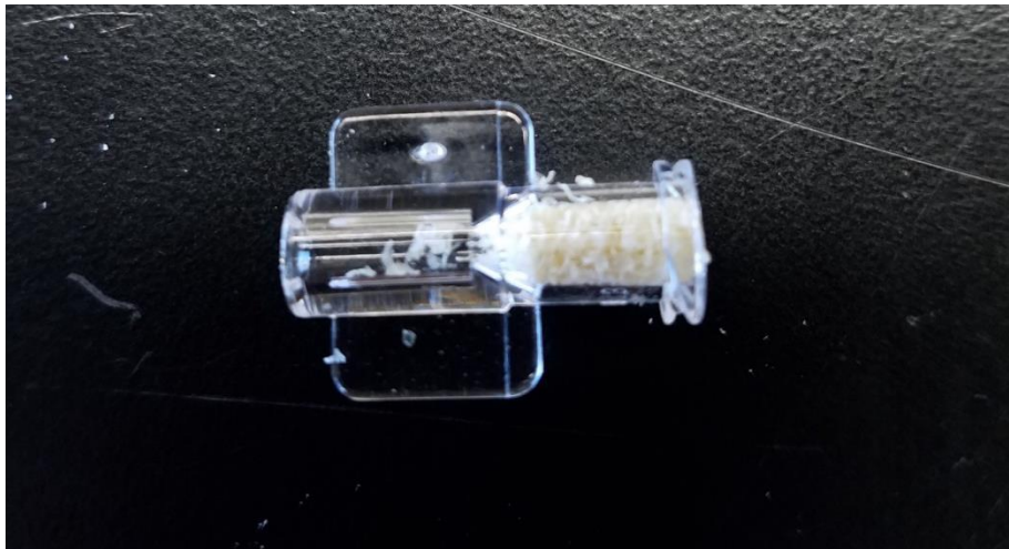
Figure 3. Powder clogged this off the shelf fitting at the stepped surface of the steep taper.
