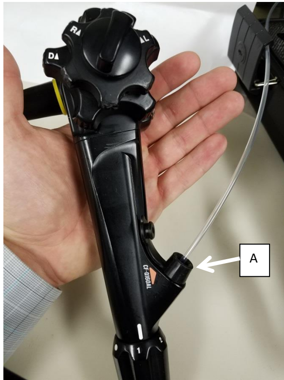
Figure 26. The final design being fed through the scope as a final functionality test. "A" calls out the biopsy cap which is a tight piece of flexible plastic through which devices are passed while maintaining insufflation pressure.
