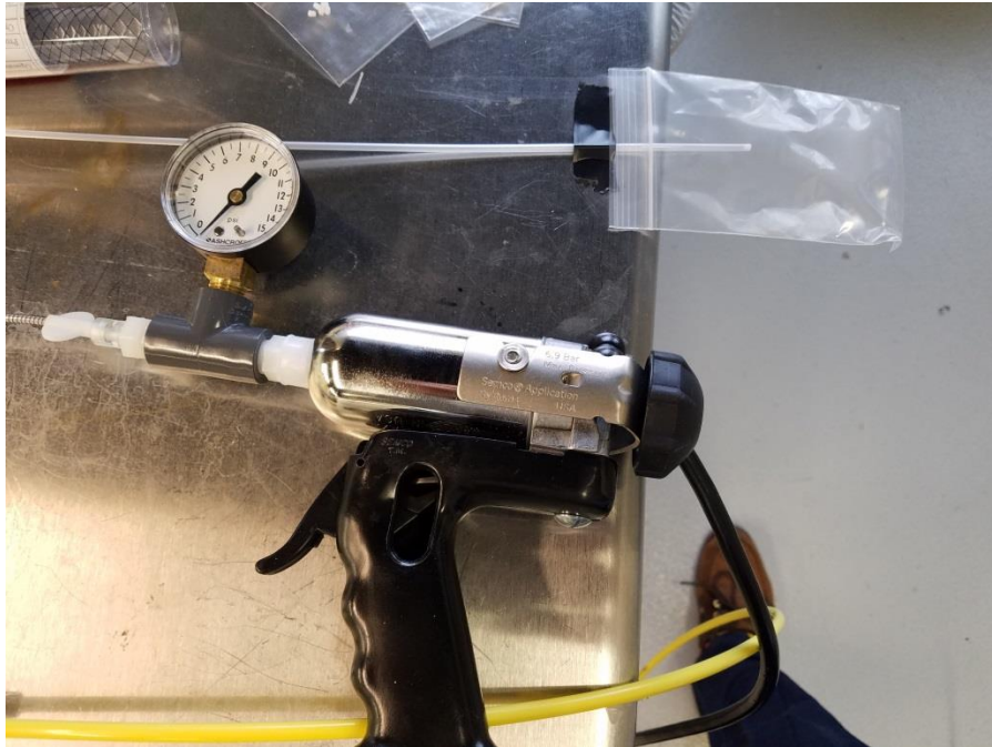
Figure 25. Setup for the end cap test with the pressure gauge and end cap close to each other to improve accuracy of results.
