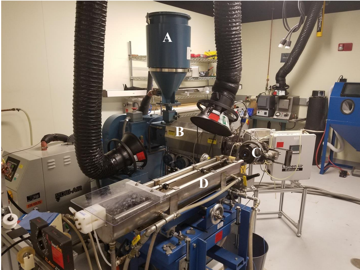
Figure 11. Commercial extruder with the hopper (A), the melting chamber (B), the location of the die (C), and the water bath (D).
