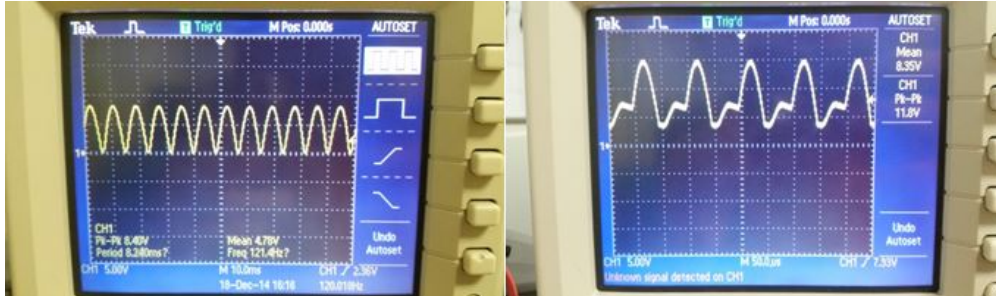
Figure 6.14: Oscilloscope view of diodes rectifying 120 Hz(left) and 10 kHz (right)
