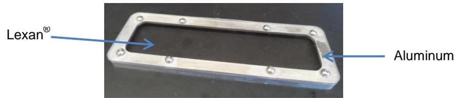
**Figure 11 – Tissue Culture Chamber Lid.** The lids for the chambers are a two-piece design constructed from Lexan<sup>®</sup> polycarbonate and aluminum.
