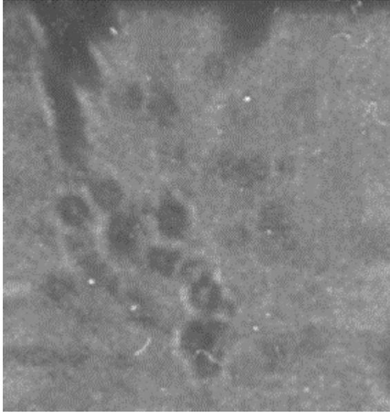
Fig. 4.4 Typical photo of droplets (large dark circles) being injected into Mach 1.8 flow. Primary flow is from left to right, droplets being injected from upper left. Actual droplet size is approximately 0.09mm (0.0035 in.).
