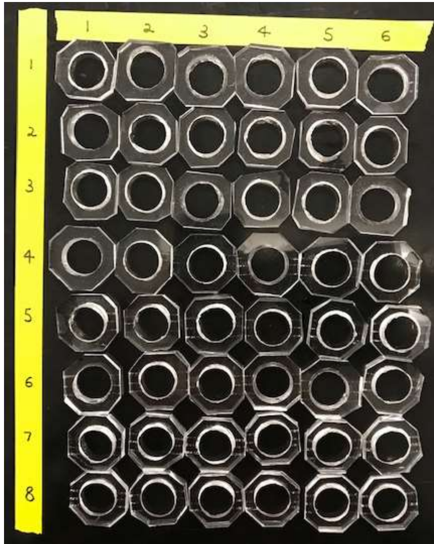
Figure 36. Pins Lab Model PDMS frames for reproducibility testing, n=48 .
