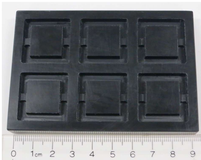
Figure 25. Machined Delrin™ acetal plastic mold
