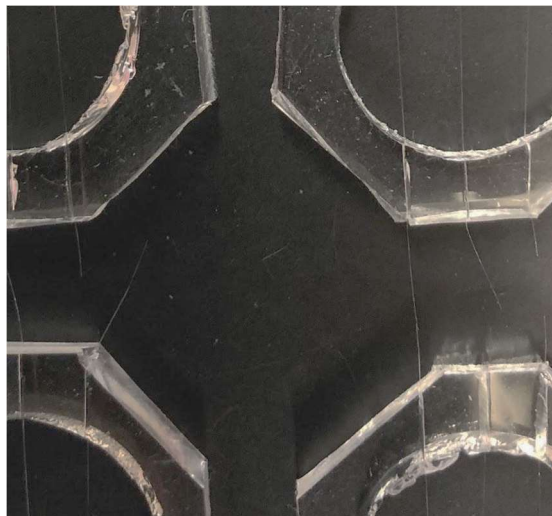
Figure 2. PDMS ring with fibrin microthreads
