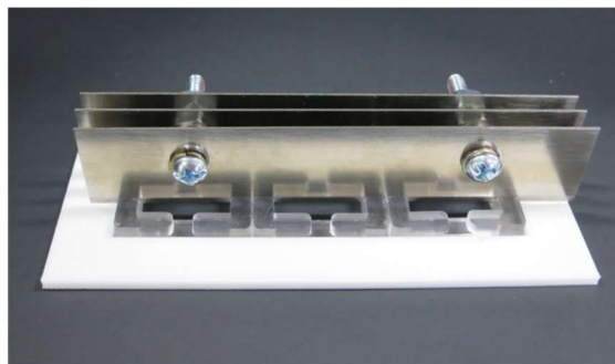
Figure 33. Steps taken to construct fibrin microthread fixation slits using cutting guide and tool
