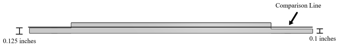
Figure 32: This figure shows the bottom of the module with measurements of the heights of both wings and a line to compare the difference in the heights of the wings. The right wings have a shorter height of 0.1 inches while the left wings have a height of 0.125 inches.
