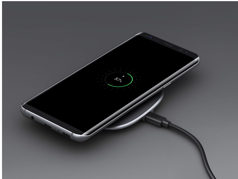
Figure 19: The power transmitter on the wireless phone charging pad is located in the pad below the phone, while the power receiver is located within the phone itself.
