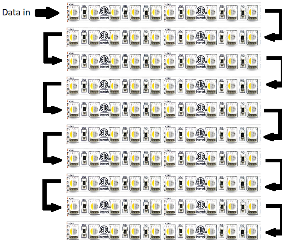
Figure 28: The power is connected in parallel while data and clock lines are connected in series as shown by the arrows.
