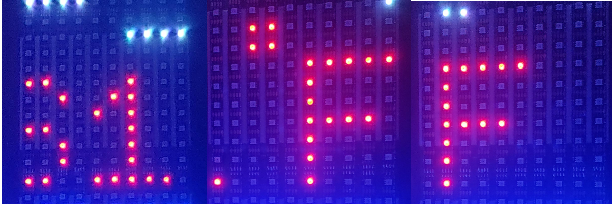
Figure 69: This animation converts a string of ASCII characters into pixel indexes on the matrix. These pixels are shifted to the right and scroll from the right edge to the left in an infinite loop.
