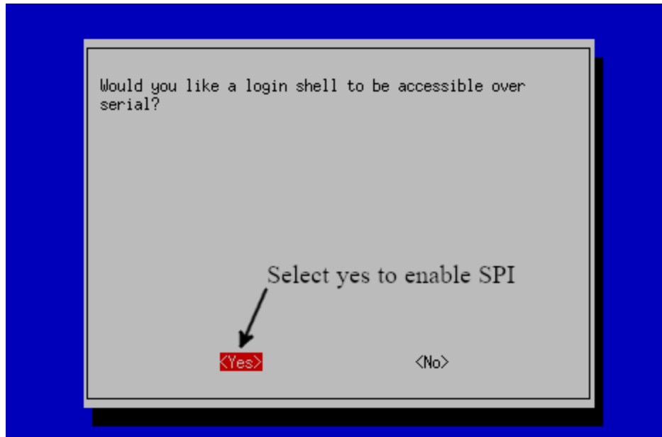
Figure 50: SPI Enable. After selecting SPI, highlight “<Yes>”. Press enter and reboot the Pi to enable SPI.
