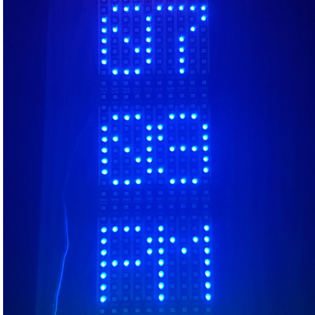
Figure 68: This animation converts a string of ASCII characters into pixel indexes on the matrix. With this, static letters are drawn and remain in place.
