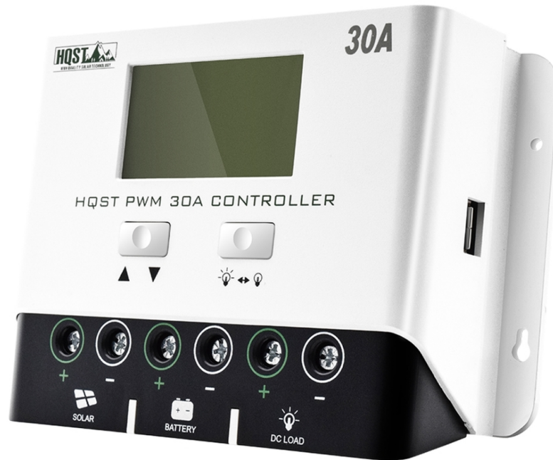
Figure 23: The charge controller features protection against several battery life shortening aspects such as battery short-circuit, over-current, overload, and overheating. Any system issues can be easily diagnosed with assistance from the system error codes and information that display on the LCD screen [40].
