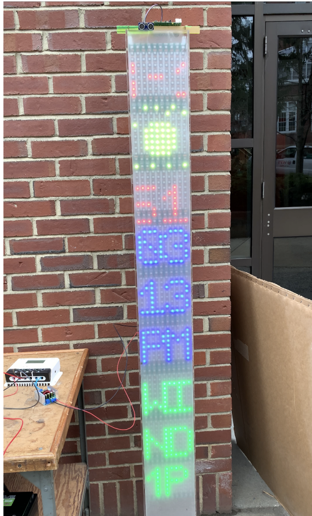
Figure 2: The display is shown outside during the live demo. It is displaying the date, time, temperature, weather, and wind speed. The Raspberry Pi and distance sensor are located at the top of the display.
